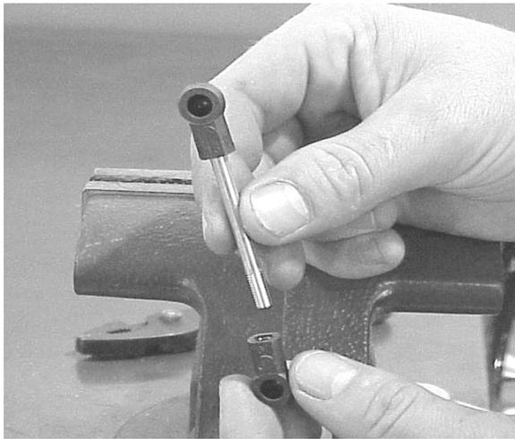
12. Locate the new Eibach sensor links (long links) and thread one ball socket onto each end. Screw the sockets down until they gently bottom out. **NOTE: Do not over tighten the sockets**
