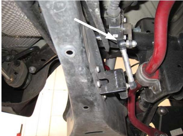
10. Reconnect the sensor link to the control arm. (See Photo 25)
