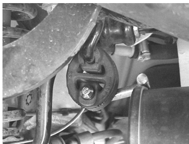
(Photo 9) Rubber exhaust hangers
