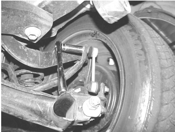
(Photo 11) Passenger end link
