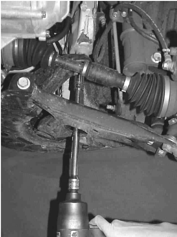
(Photo 4) Front sub frame bolt
