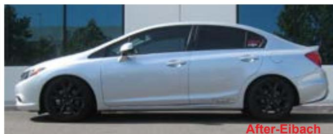
**Please note:** spring rates are measured as a system of the front or rear suspension. 10 mm of bump-stop deflection is included in the final rate of the system. Lowering numbers are based on sedan model.
