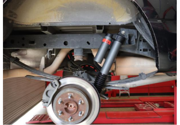
(RIGHT SIDE- PASSENGER) shown above with reservoir facing axle/rear of vehicle.
