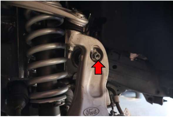
19. Reinstall the sway bar end link nut using an 18mm socket and tighten to manufacturer specification.
