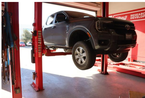
1. Lift the vehicle and remove the front wheels.
