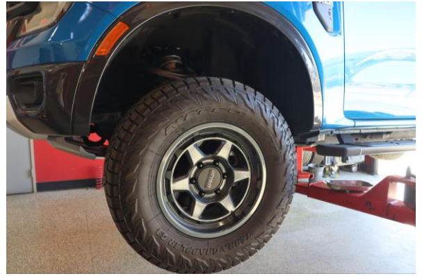
20. Install the wheel and tire using a 19mm socket, tighten to manufacturer specification.
