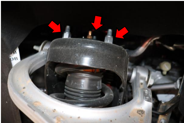
9. Remove the three 15mm top hat nuts.
