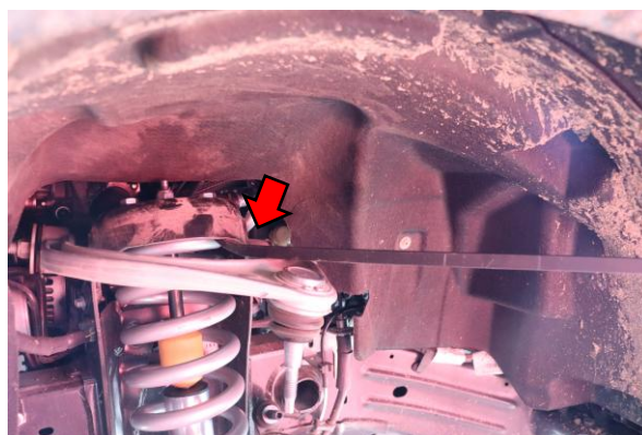
6. Use a pry bar to pull down on the upper control arm. Remove the upper ball joint nut and slowly allow the upper control arm to lift out of the steering knuckle.
