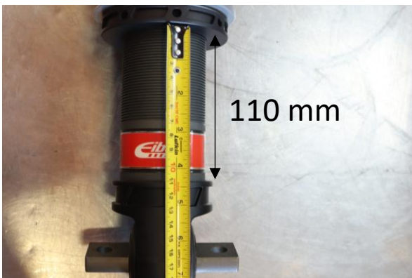
11. Verify pre-load of the coilover by measuring from the bottom of the lower spring perch to the top of the lower shock mount. Out of the box this setting should be 110mm which will provide a ride height level with the OE rear suspension. Exceeding 3" of lift may result in poor ride quality.
