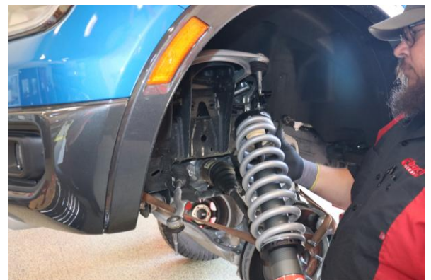
12. Install the Eibach Pro Truck Coilover 2.5 into the vehicle.
