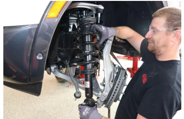
10. Remove the OEM shock assembly from the vehicle.
