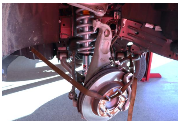
4. Use a strap to hold the rotor and steering knuckle against the vehicle. This will help prevent damage to the front axle due to overextending.
