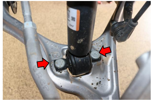
8. Use hammer to drive out both lower shock mount studs from the bottom. Applying heat to the studs can assist in their removal, be careful not to overheat the surrounding bushing or shock body.
