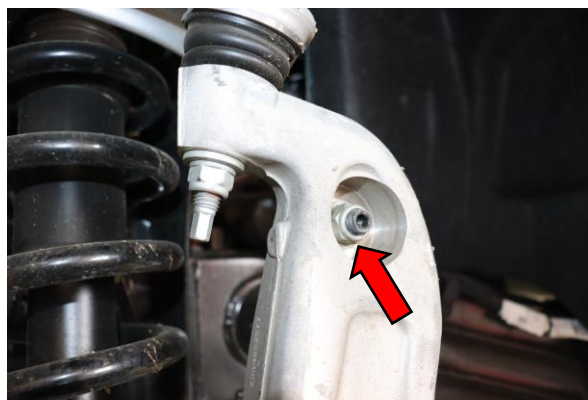
2. Remove 18mm sway bar end link.
