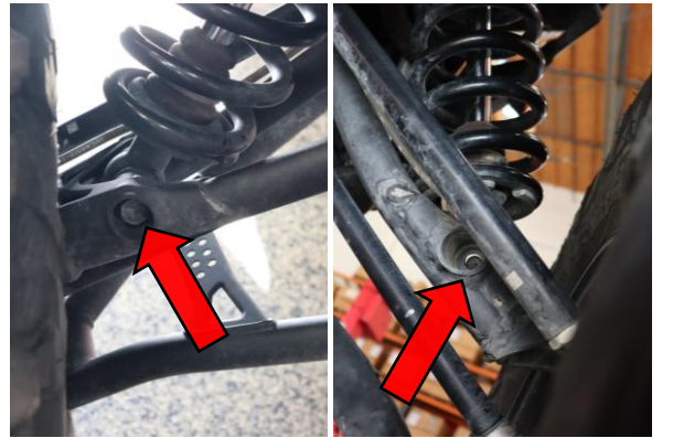
Step 4. Use two 18mm to remove the lower shock mount nut and bolt.
