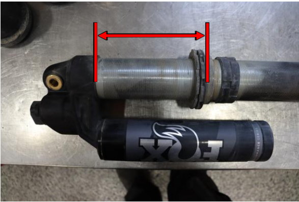
Step 9. Set pre-load of spring seat to 80mm (3 1/8in.) from bottom of seat to bottom of reservoir bridge.
