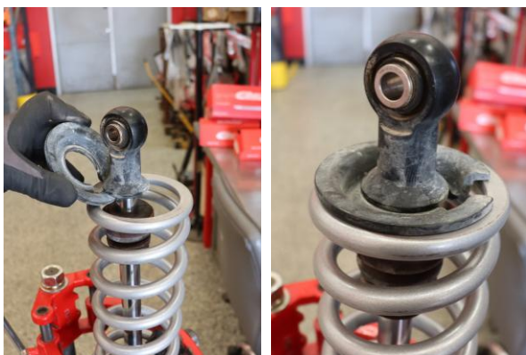
Step 15. Compress spring assembly enough to install lower spring perch. Decompress shock and ensure spring and perch sit flush on the lower mount.
