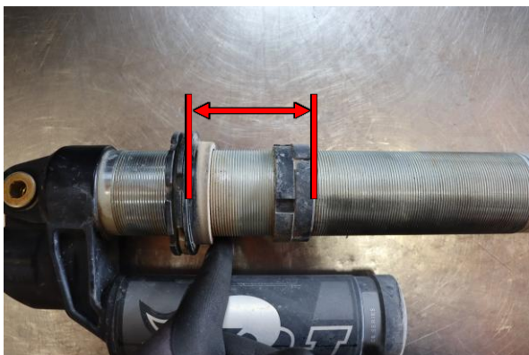
Step 11. Set the crossover ring to 85mm (3 3/8in.) from the bottom of the spring seat to the bottom of the crossover ring.
