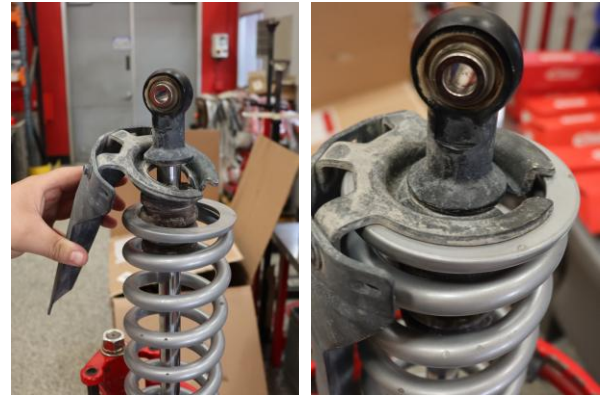
Step 14. Compress the spring assembly and install the lower spring perch. Decompress the spring assembly making sure that the lower spring perch seats completely against the lower shock mount.
