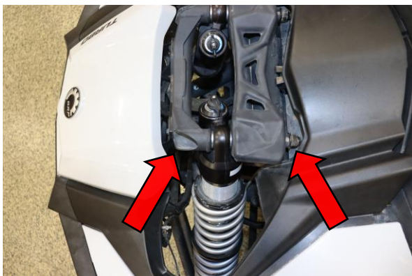
Step 17. Use two 18mm to install and tighten the upper shock mount nut and bolt to manufacturer specification.
