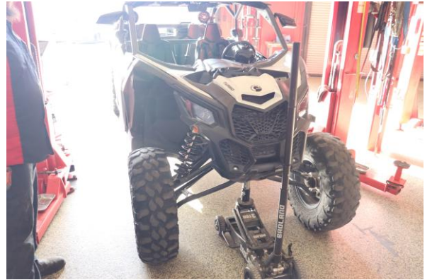
Step 2. Lifting only enough to allow the wheel to spin freely will help ease removal, installation, and prevent damage to the axle from over extension.
