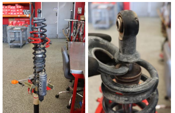
Step 6. Use spring compressor to compress the spring assembly. Remove the lower spring perch.
