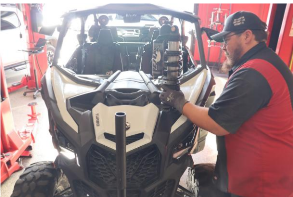
Step 5. Remove the shock assembly from the vehicle.
