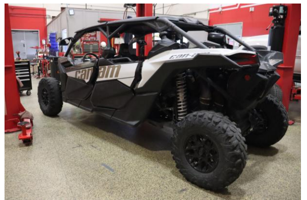
Step 18. Lower the rear of the vehicle and carefully test drive while listening for any abnormal noises.
