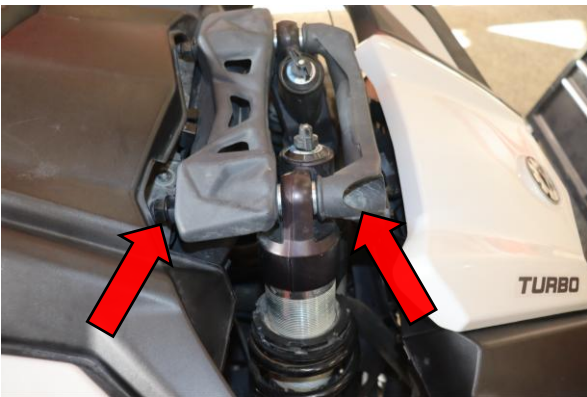
Step 3. Use two 18mm to remove the upper shock mount nut and bolt.
