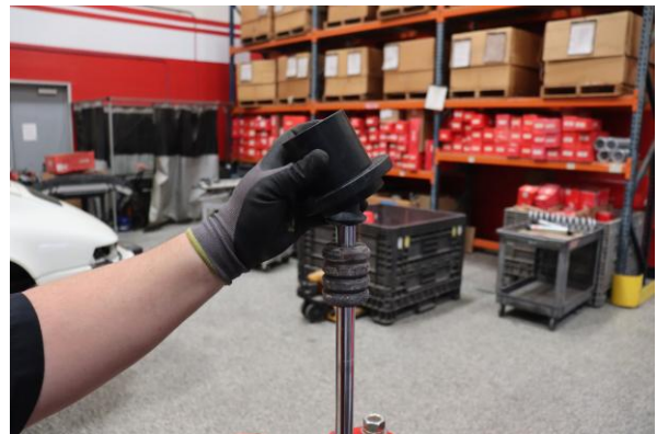
Step 12. Install the Eibach spring slider.
