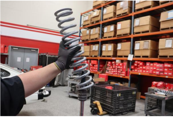
Step 13. Install the Eibach main spring.
