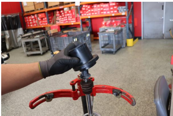
Step 13. Install the Eibach spring slider.
