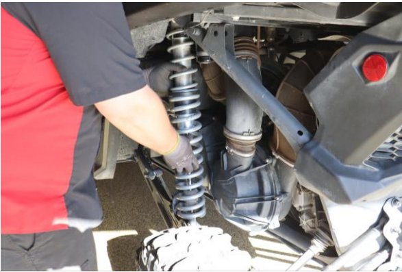
Step 15. Install the shock assembly in the vehicle.
