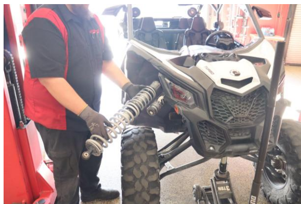
Step 16. Install the shock assembly in the vehicle.
