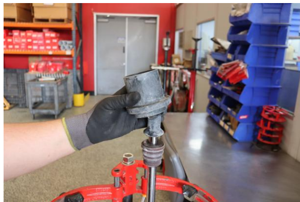
Step 8. Remove the OE spring slider.
