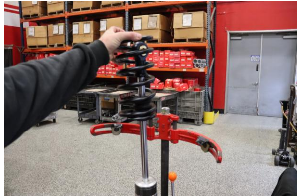
Step 10. Remove the OE rear secondary spring.
