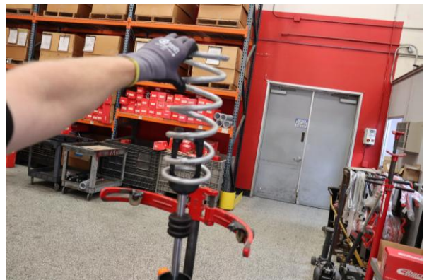
Step 18. Install the Eibach front main spring.
