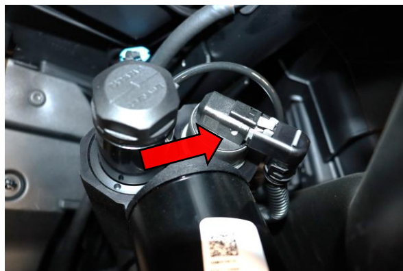
Step 21. Reconnect both compression and rebound electrical connectors.
