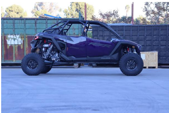
Step 22. Lower the vehicle and carefully test drive while listening for any abnormal noises. Measure from the ground to the center of the skid plate between the rear mount of the front lower control arms. The recommended preload measurement in Step 13 will get the vehicle close to the recommended ride height but each vehicle may vary some. We recommend setting the ride height at 485mm (16.75in.) measuring from the ground to the center of the front skid plate/ ground clearance. Note: Measurements were taken from a vehicle with 32in. tires. If your vehicle has a different size tire, the ride height will need to be adjusted. Due to the sensitivity of weight of these vehicles, weight distribution may change ride heights, additional pre-load may need to be added to compensate.
