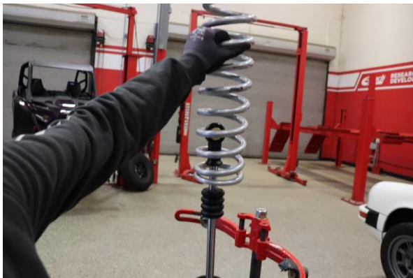
Step 17. Install the Eibach rear main spring.
