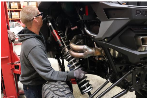
Step 19. Install the shock assembly in the vehicle.
