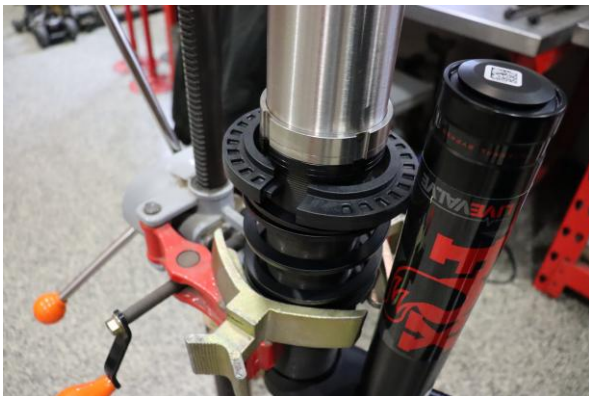
Step 11. Remove the second OE rear spring slider.
