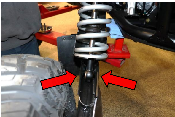
Step 21. Use two 21mm to install the lower shock mount nut and bolt. Tighten to manufacturer specification.
