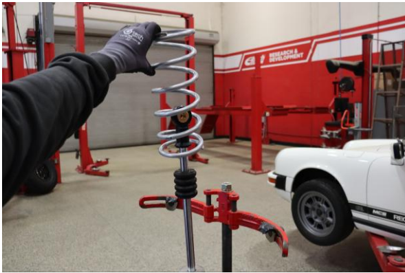
Step 15. Install the Eibach rear secondary spring.
