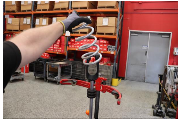
Step 16. Install the Eibach front secondary spring.
