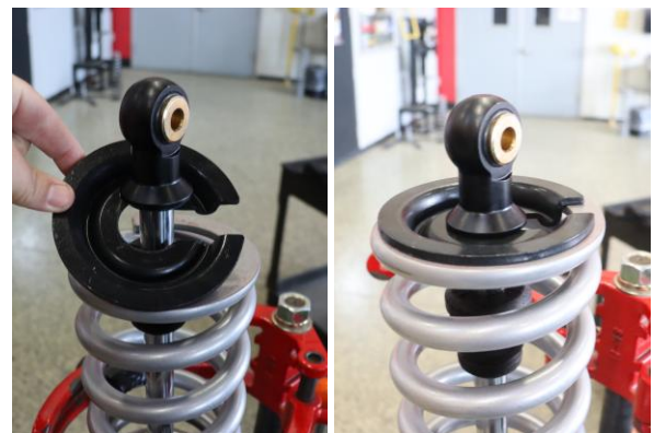
Step 18. Use a spring compressor to compress the spring assembly. Install the OE lower spring perch. Slowly decompress the spring assembly. Ensure that the lower spring perch seats full against the lower shock mount.
