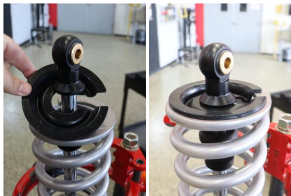
Step 18. Use a spring compressor to compress the spring assembly. Install the OE lower spring perch. Slowly decompress the spring assembly. Ensure that the lower spring perch seats full against the lower shock mount.
