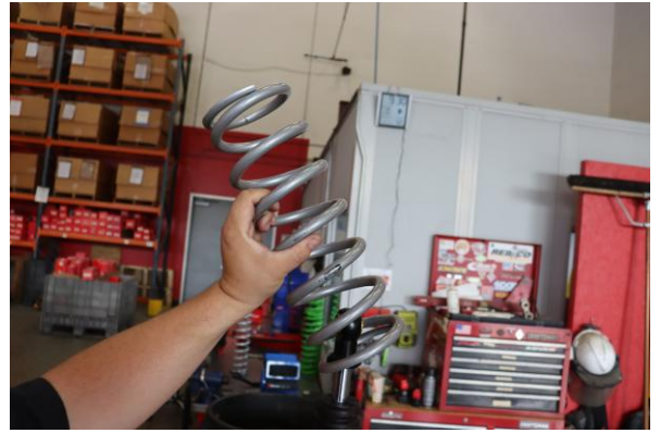
Step 14. Install the Eibach rear secondary spring.
