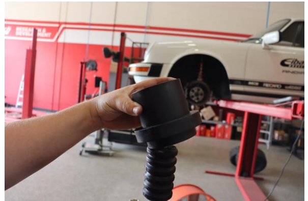
Step 10. Remove the OE rear spring slider.
