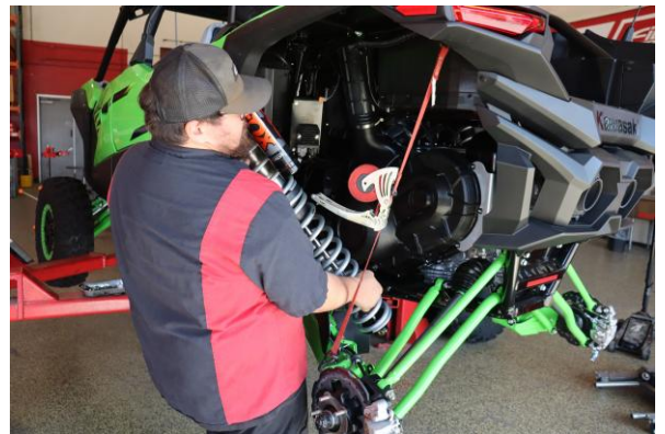
Step 18. Install the shock in the vehicle.
