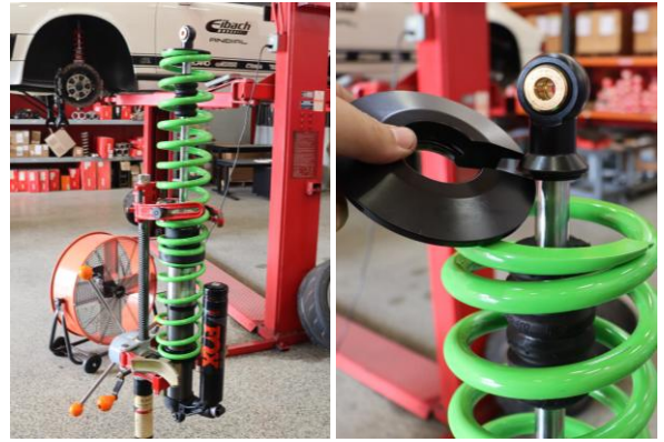
Step 8. Use a spring compressor to compress the spring assembly enough that the lower spring perch can be removed. Decompress the spring assembly.
