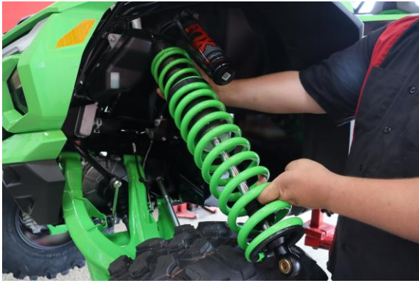
Step 7. Remove the shock from the vehicle.
