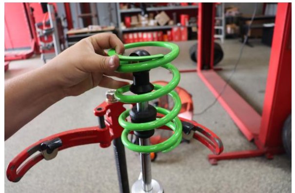
Step 12. Remove the OE front secondary spring.
