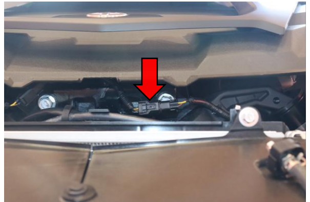
Step 22. Reconnect the shock electrical connector.
