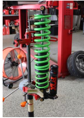
Step 8. Use a spring compressor to compress the spring assembly enough that the lower spring perch is clear of the lower shock mount.
