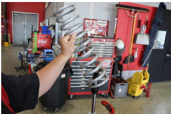
Step 17. Install the Eibach front main spring.
