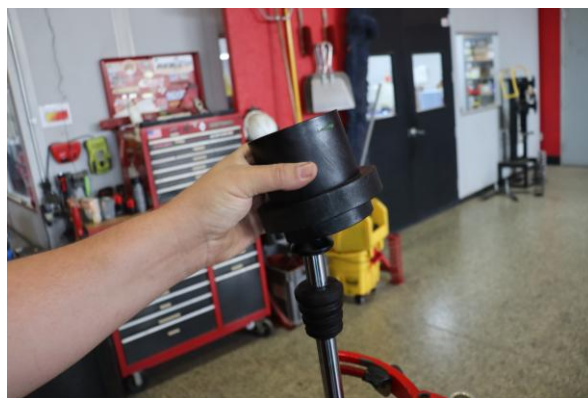
Step 16. Install the OE front spring slider.
