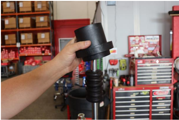
Step 15. Install the OE rear spring slider.
