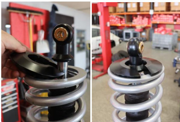
Step 17. Install the lower spring perch and decompress the spring assembly. Ensure the lower spring perch seats fully against the lower shock mount.
