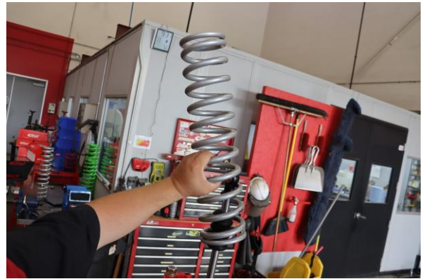
Step 16. Install the Eibach rear main spring.
