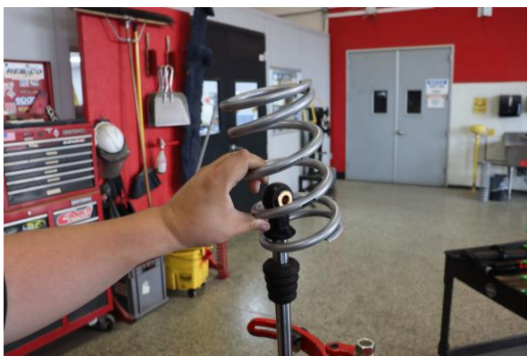
Step 15. Install the Eibach front secondary spring.
