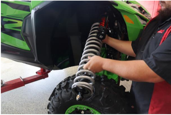
Step 19. Install the shock in the vehicle.
