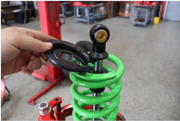
Step 9. Remove the lower spring perch and decompress the spring assembly.
