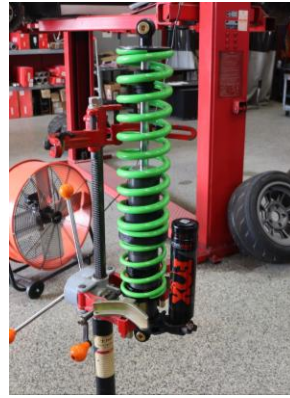
Step 8. Use a spring compressor to compress the spring assembly enough that the lower spring perch is clear of the lower shock mount.
