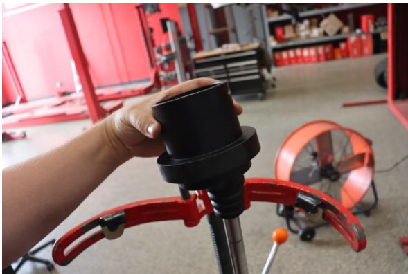
Step 11. Remove the OE front spring slider.
