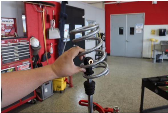
Step 15. Install the Eibach front secondary spring.
