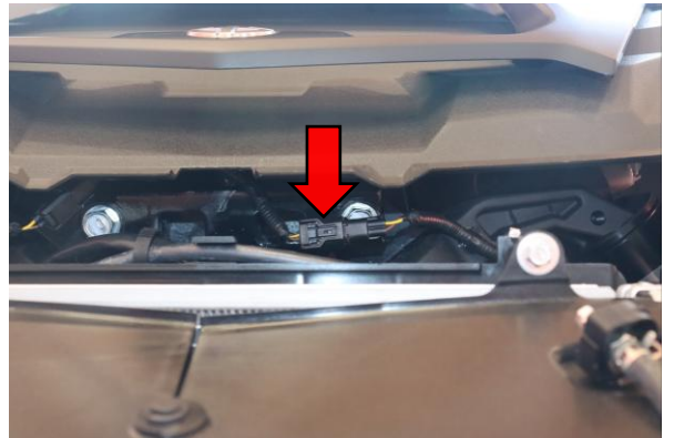
Step 22. Reconnect the shock electrical connector.
