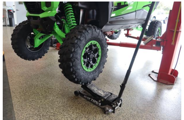
Step 24. Remove the wheel support and lower the vehicle.
