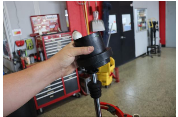
Step 16. Install the OE front spring slider.
