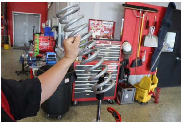
Step 17. Install the Eibach front main spring.
