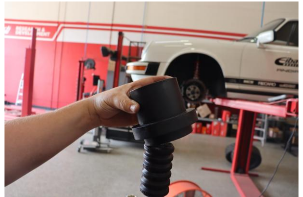
Step 10. Remove the OE rear spring slider.
