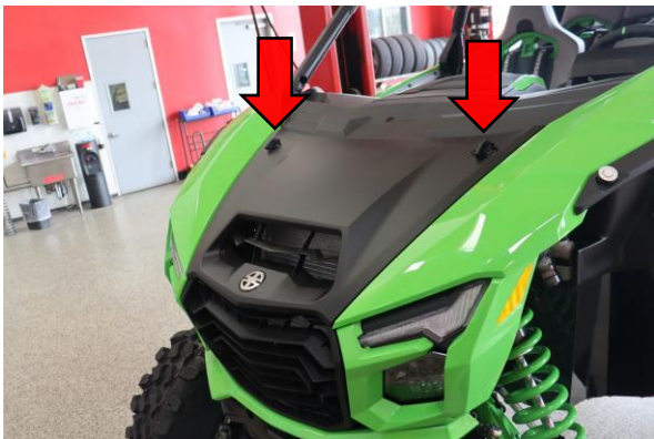
Step 23. Reinstall the hood and secure by turning both latches 90 degrees.
