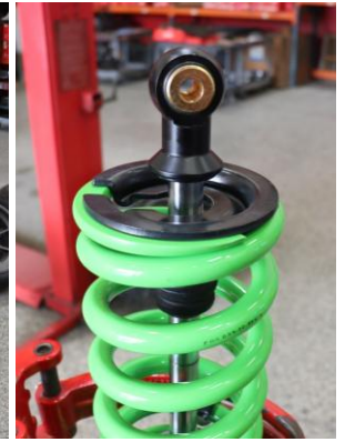
Step 8. Use a spring compressor to compress the spring assembly enough that the lower spring perch is clear of the lower shock mount.
