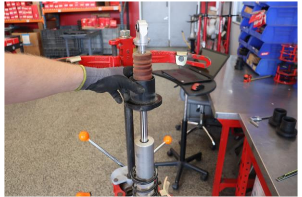
Step 10. Remove the first OE spring slider.
