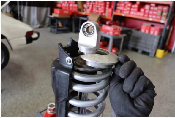
Step 19. Install the OE lower spring perch.
