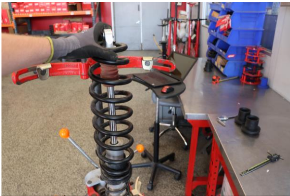
Step 9. Remove the OE main spring.
