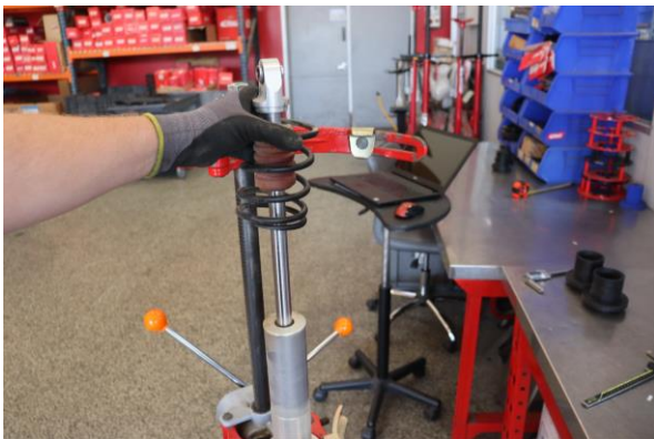
Step 11. Remove the OE tender spring.
