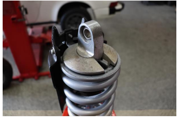
Step 20. Decompress the shock assembly ensuring the lower spring perch fully engages the lower shock mount.
