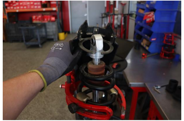
Step 8. Remove the OE plastic shield.
