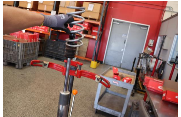
Step 16. Install Eibach front secondary spring.
