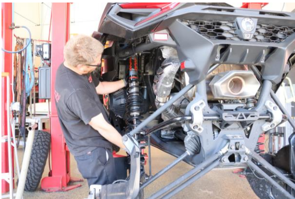
Step 5. Rotate the top of the shock assembly to the rear of the vehicle enough to clear the mount. Lift assembly from the bottom to clear the rear trailing arm and remove shock assembly from the vehicle.
