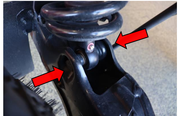
Step 4. Remove 21mm lower shock nut and bolt. (This bolt from the manufacturer has a yellow Loctite that may require a large breaker bar to remove).
