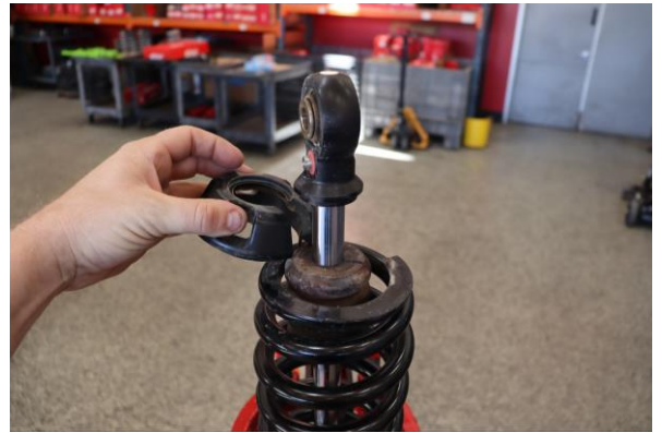
Step 10. Remove the lower spring retainer.
