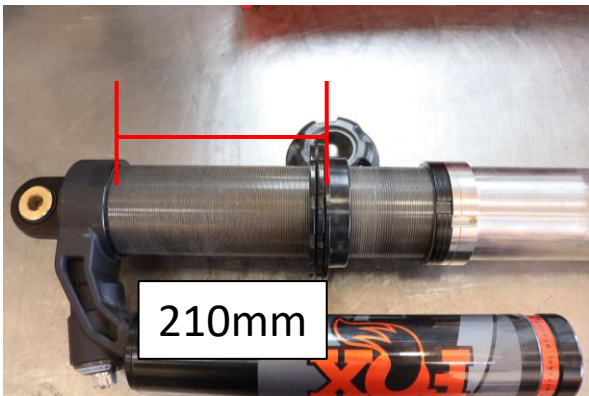
Step 11. Set pre-load to 210mm (8 17/64 in.) from bottom of spring seat to bottom of furthest point on reservoir bridge. (Reservoir bridge is not flat relative to spring seat. Be sure to measure from the side opposite the reservoir).
