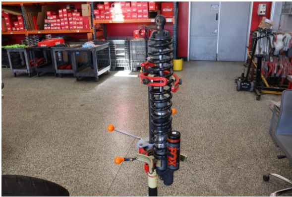
Step 9. Use spring compressor to compress shock assembly.
