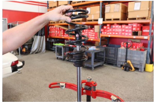
Step 10. Remove OE secondary spring.
