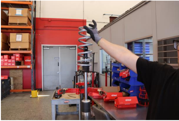
Step 13. Install Eibach secondary spring.
