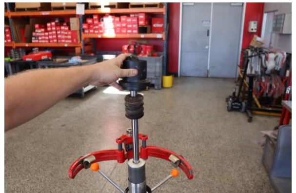
Step 12. Remove OE slider.
