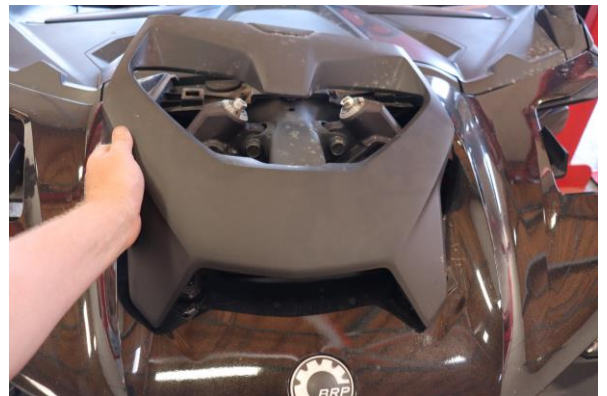
Step 24. Reinstall cover on front of car.
