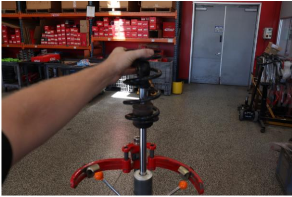
Step 13. Remove OE secondary spring.
