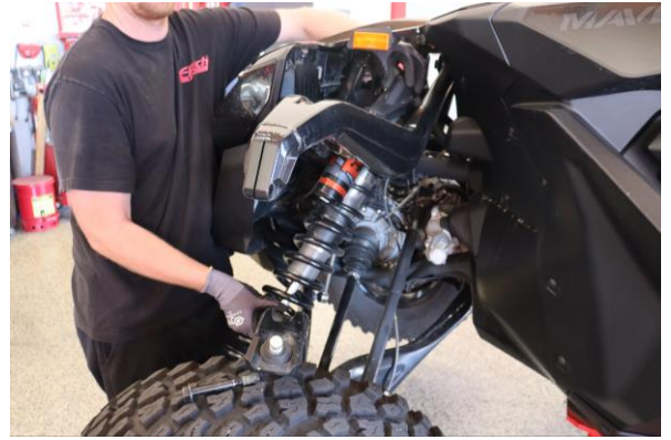
Step 8. Remove lower shock from mount first toward front of car.
