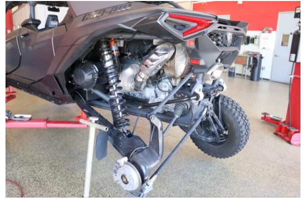
Step 2. Remove wheel and tire. Secure trailing arm to frame using strap. Note: Never work on or under a vehicle that is not supported by the proper safety equipment.
