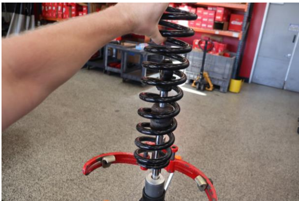
Step 11. Remove OE front main spring
