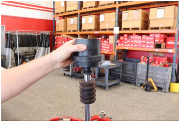
Step 9. Remove OE spring slider.
