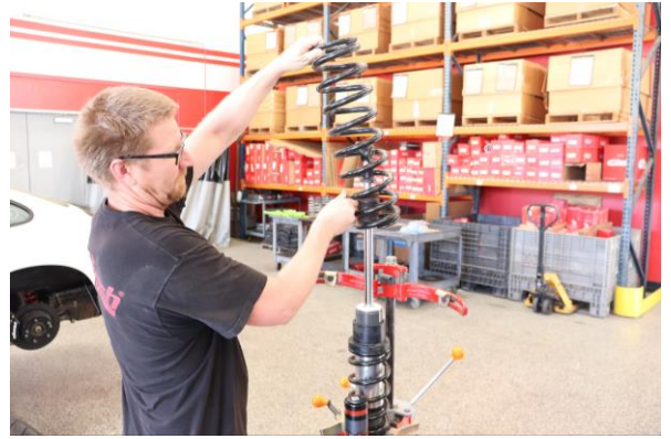
Step 8. Remove OE main spring
