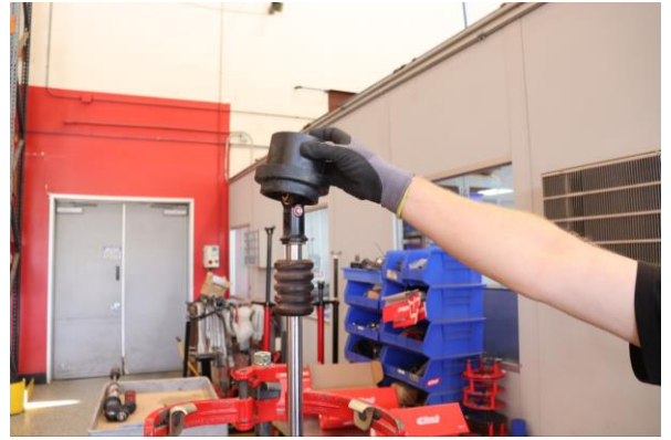
Step 14. Reinstall OE spring slider.
