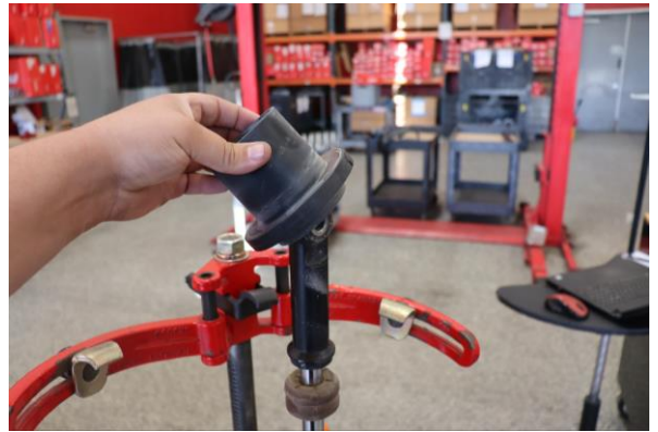
Step 16. Install spring slider.
