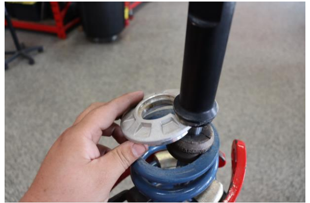
Step 10. Remove the lower spring perch.
