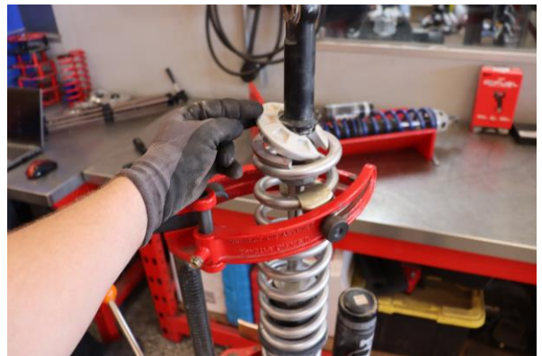
Step 18. Install the lower spring perch. Decompress the shock assembly and check to make sure the spring perch is fully engaged.
