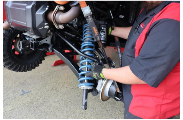
Step 8. Lift slightly on the wheel hub to remove the upper and lower shock mount bolts. Rotate the top of the shock out of the upper mount and lift out of the lower mount. Remove the shock assembly between the upper and lower control arm.
