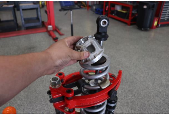
Step 15. Compress the spring assembly and install the lower spring perch.
