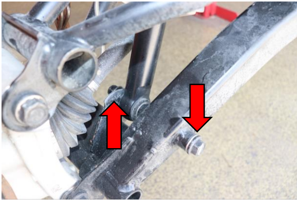
Step 21. Use two 18mm to install the lower shock mount nut and bolt. Tighten to factory specification.
