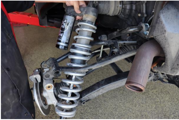
Step 19. Place the rear shock assembly in the vehicle by inserting between the upper and lower control arm.
