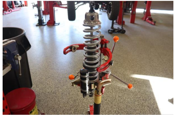
Step 16. Decompress assembly and ensure lower spring perch engages lower shock mount fully.
