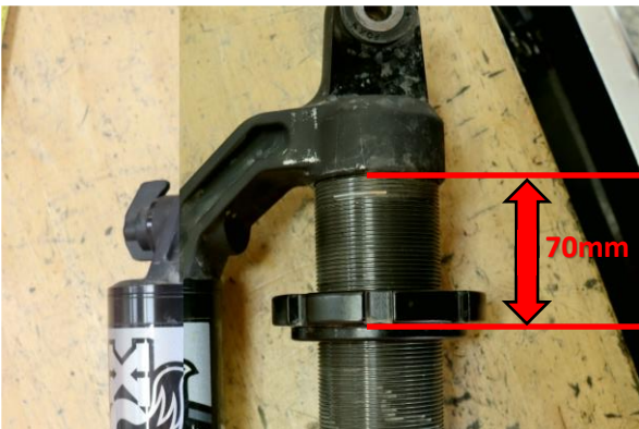
Step 11. Remove shock from the spring compressor. Adjust the upper spring perch to 70mm (2 3/4in) measuring from the spring seat to the bottom of the bridge to set spring preload.
