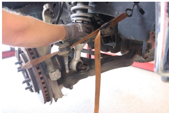
8. Use straps to hold steering knuckle from damaging front axles.
