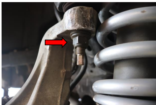
9. Remove 18mm nut from UCA ball-joint to steering knuckle and use hammer to separate the arm from knuckle.
