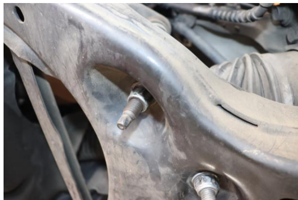
20. Install hardware for sway bar end link to lower control arm 18mm. OE torque spec (62 lb-ft)
