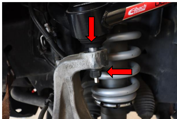
18. Install upper control arm to steering knuckle use supplied washer between nut and knuckle. OE torque spec (85 lb-ft)
