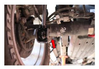
11. Install 15mm lower shock bolt and tighten to manufacturer specification of **59ft.lbs**.
