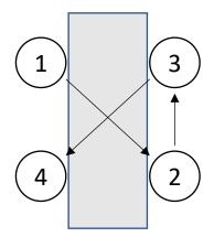
Tightening in a cross pattern is critical and failure to do so may result in suspension failure.
