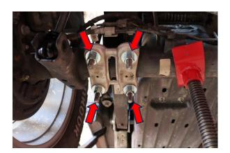
10. Install the supplied 21MM nuts and washer on the U-bolts. Tighten to **100ft.lbs.** using an X pattern.
