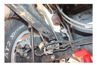
8. Install the supplied longer U-bolts over the top of the leaf spring.
