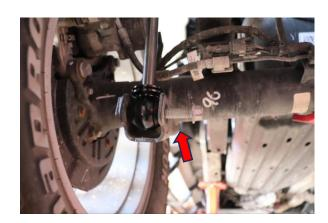
4. Remove 15mm lower shock bolt.
