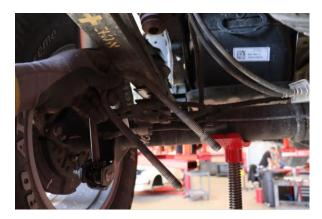
5. Remove both U-bolts from the top of the leaf spring.
