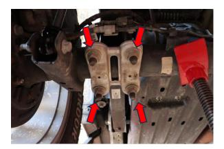
2. Remove four 21mm U-bolt nuts.
