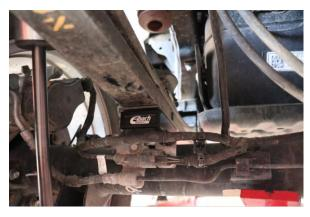
7. Install the Eibach lift block with the pin facing down. Lift the axle making sure the bottom pin of the leaf spring seats inside the lift block and the lift block pin seats inside the axle.
