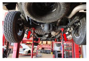
1. Lift and support the vehicle. **Note: Never work on or under a vehicle that is not supported by the proper safety equipment.** Use jacks to support the rear axle.
