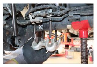
9. Reinstall the OE axle clamp on the supplied U-bolts.
