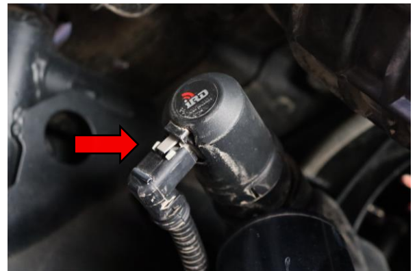
Step 24. Reconnect the shock electrical connector.
