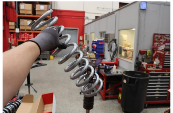
Step 18. Install the Eibach main spring.
