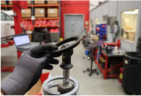
Step 19. Install the supplied Eibach spring adapter on the main spring.
