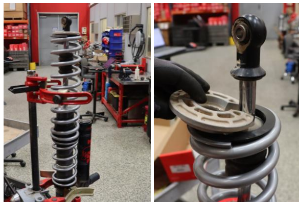
Step 20. Use a spring compressor to compress the spring assembly. Install the lower spring perch. Slowly decompress the shock assembly making sure that the lower spring perch full seats against the lower shock mount.
