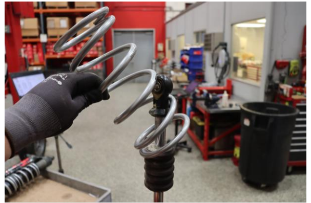
Step 16. Install the Eibach secondary spring.
