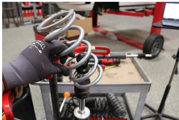
Step 14. Install the Eibach secondary spring.
