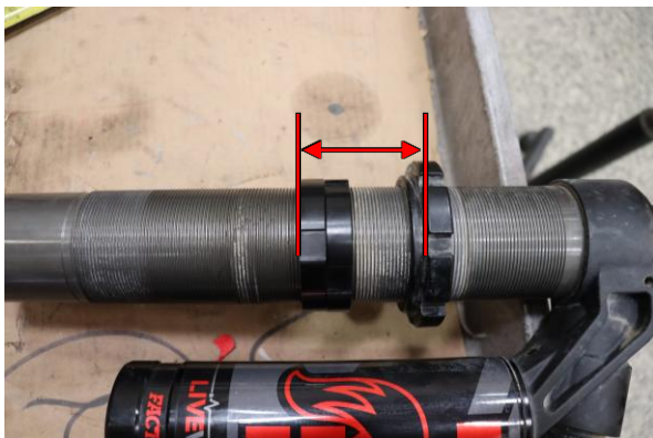
Step 13. Install the Eibach crossover rings. Adjust rings to be 60mm (2 3/8") from the bottom of the rings to the spring seat.
