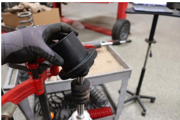
Step 15. Install the Eibach spring slider with the larger end facing away from the secondary spring.
