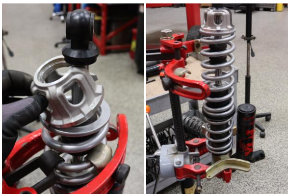
Step 17. Use a spring compressor to compress the shock assembly. Install the lower spring perch. Slowly decompress the shock assembly making sure that the lower spring perch fully seats against the lower shock mount.
