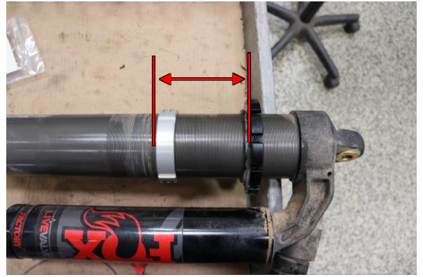
Step 14. Adjust the Eibach supplied crossover ring to 100mm (3 15/16") from bottom of spring seat to bottom of crossover ring.
