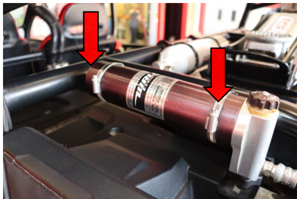
Step 25. Install reservoir and tighten clams
