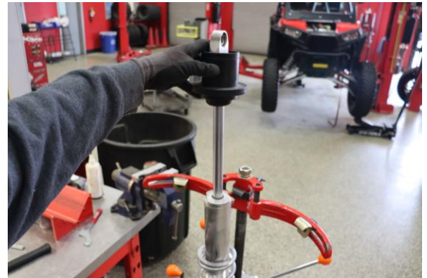
Step 10. Remove the first OE spring slider.
