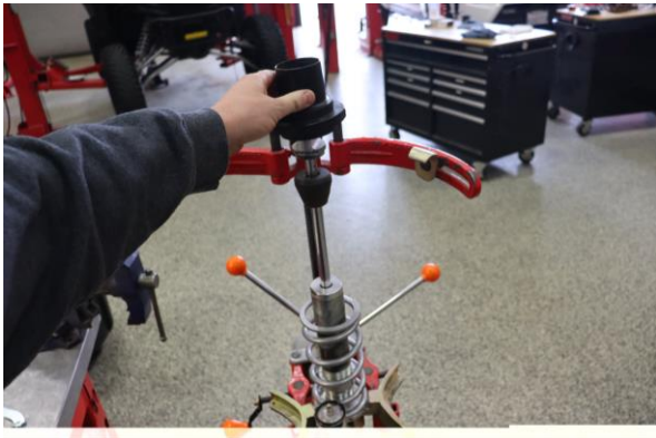
Step 9. Remove the OE spring slider.
