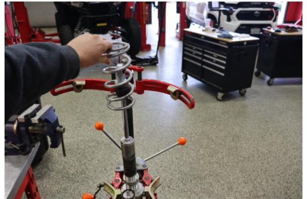
Step 10. Remove the OE tender spring.
