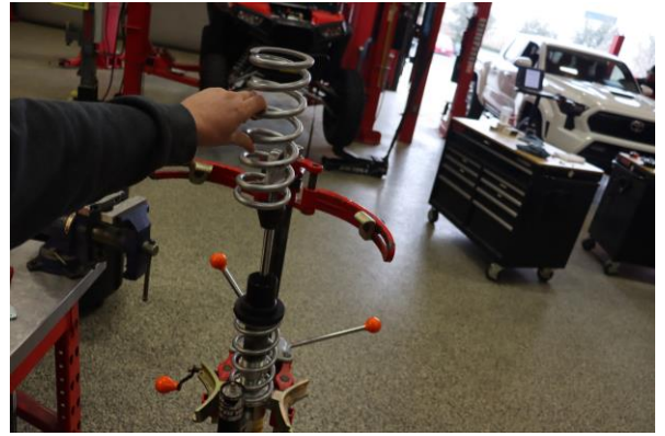
Step 8. Remove the OE main spring.
