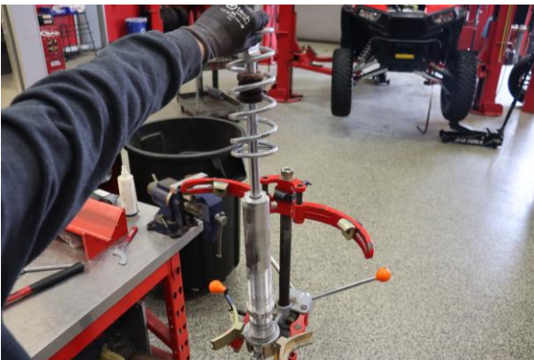
Step 11. Remove the OE tender spring.
