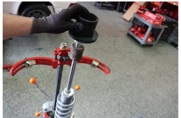
Step 16. Install Eibach spring slider with the short end facing the top of the shock.
