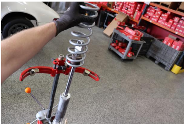
Step 15. Install Eibach tender spring.
