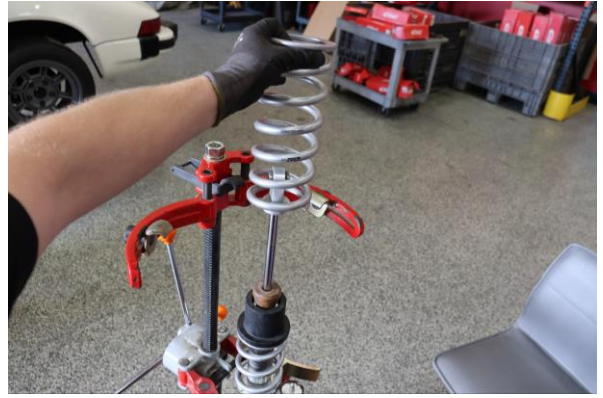
Step 14. Install Eibach main spring. Compress the spring assembly.
