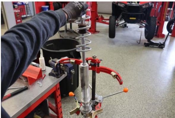
Step 11. Remove the OE tender spring.
