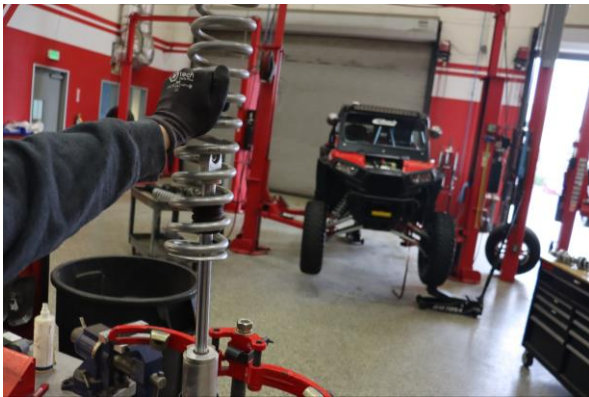
Step 9. Remove the OE main spring.
