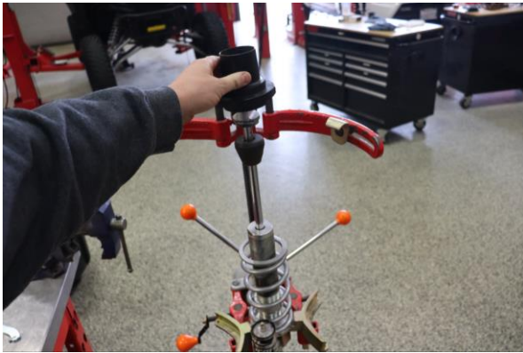
Step 9. Remove the OE spring slider.
