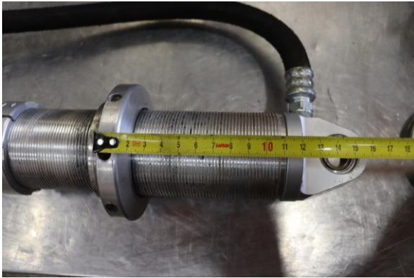
Step 13. Set pre-load to 115mm (4 ½") from bottom of spring seat to bottom of reservoir bridge collar.
