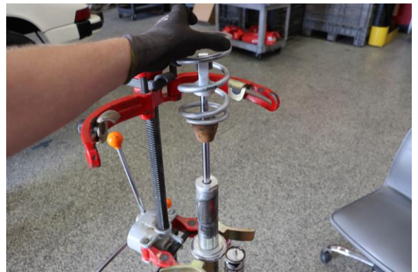
Step 12. Install Eibach front tender spring
