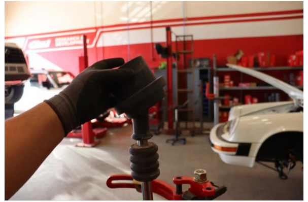
Step 8. Remove the rear spring slider.
