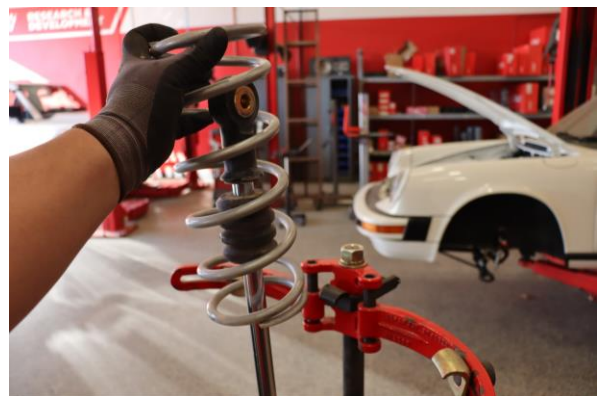
Step 12. Install Eibach rear secondary spring.
