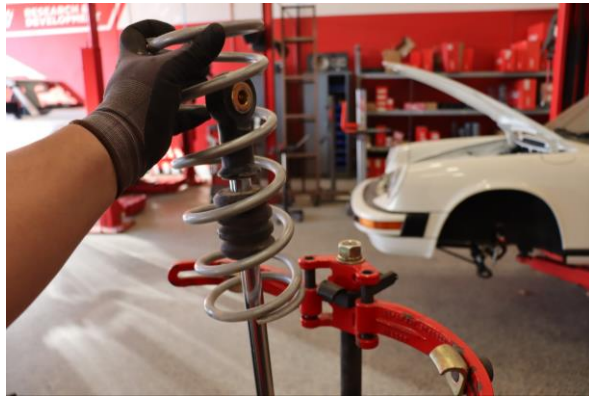
Step 9. Remove the rear secondary spring.
