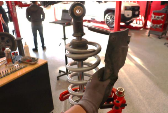
Step 15. install the lower spring perch. Decompress the spring assembly ensuring that the lower spring perch properly engages the lower shock mount. The rock guard should face the opposite direction of the reservoir at the top of the shock.
