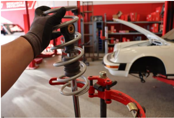
Step 9. Remove the rear secondary spring.
