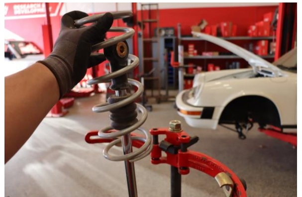
Step 12. Install Eibach rear secondary spring.
