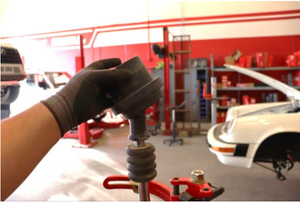
Step 13. Install the spring slider with the large end facing away from the secondary spring.
