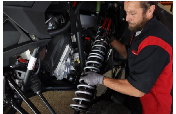
Remove the shock assembly and remove the stock springs.
