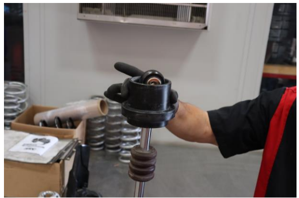
Install the OE slider the Eibach main spring.
