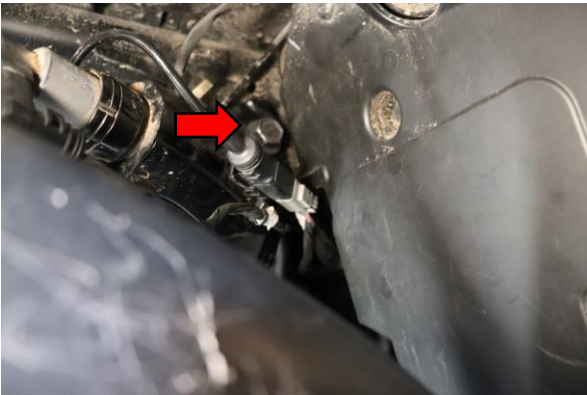
Remove the upper shock bolt with a 21mm socket.
