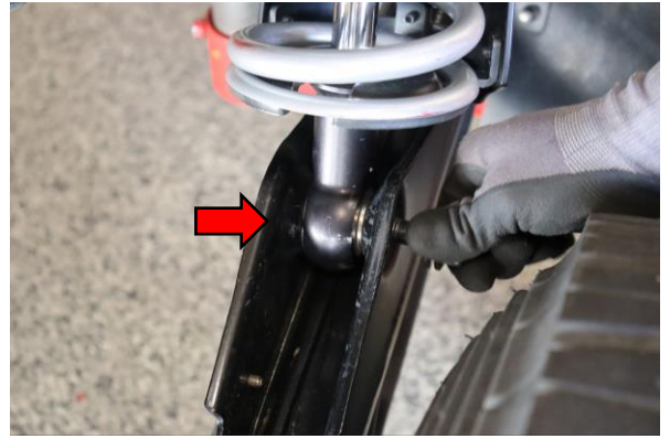
Remove the lower shock bolt with a 21mm socket.
