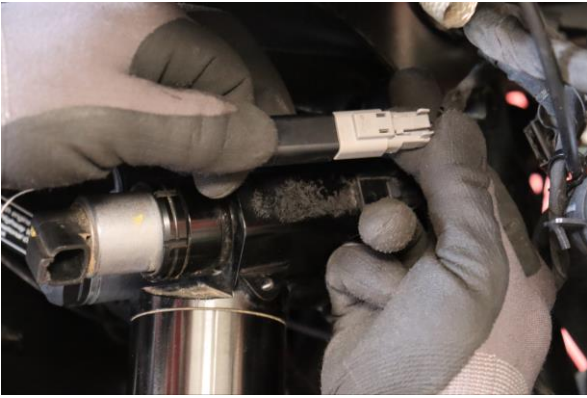
Unplug both connectors on each of the rear shocks.
