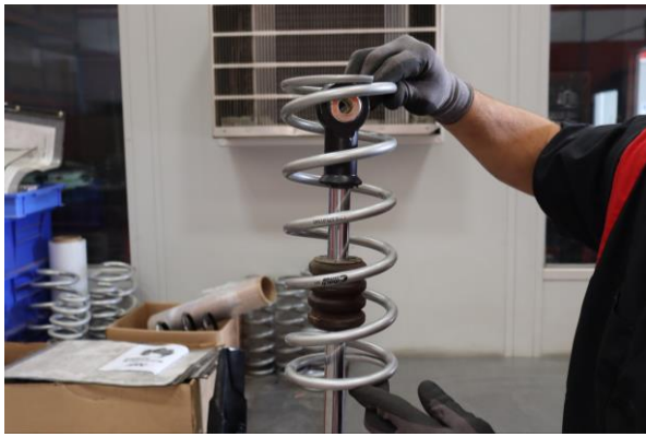
Install the Eibach secondary spring.
