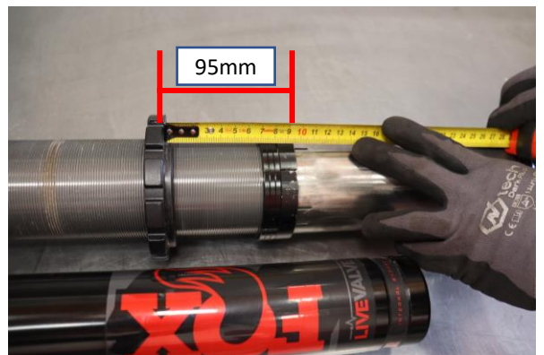
Set the crossover ring to 95mm (3 3/4in.) from the bottom of the spring seat to the bottom of the crossover rings.
