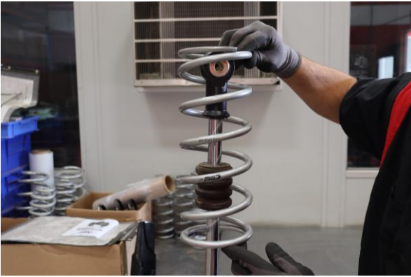
Install Eibach secondary spring
