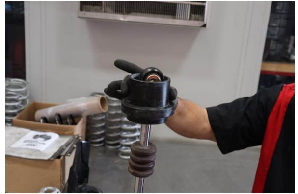
Install OE slider and Eibach main Spring
