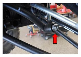
Step 1. Remove upper sway bar end link nut and bolt on both the left and right side of the vehicle.
