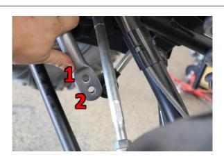
Step 6. Install the sway bar end link using 15mm.
