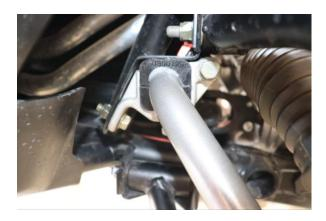
Step 5. Grease the inside of the Eibach sway bar bushings. Install Eibach sway bar bushings using OE brackets using supplied hardware.
