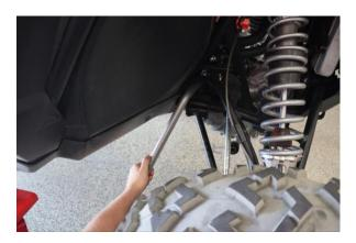
Step 4. Install the Eibach rear sway bar using the same orientation.
