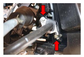
Step 2. Remove two left and two right sway bar bracket bolts.
