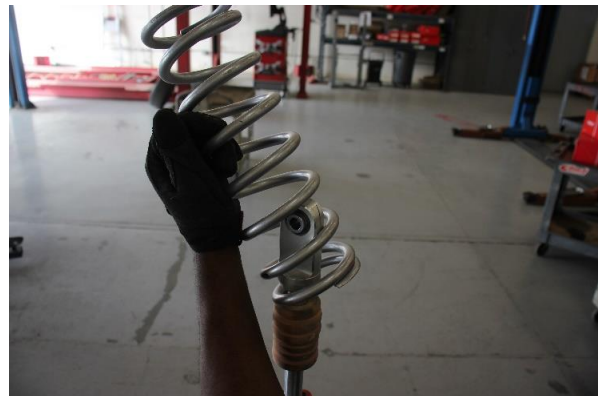
Step 12. Install the Eibach secondary spring.
