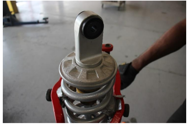
Step 14. Compress the spring assembly and re-install the spring retainer.
