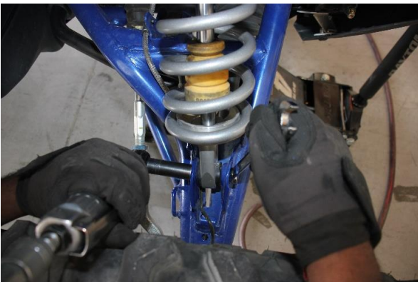
Step 17. Secure the coilover to the control arm using the OE hardware.
