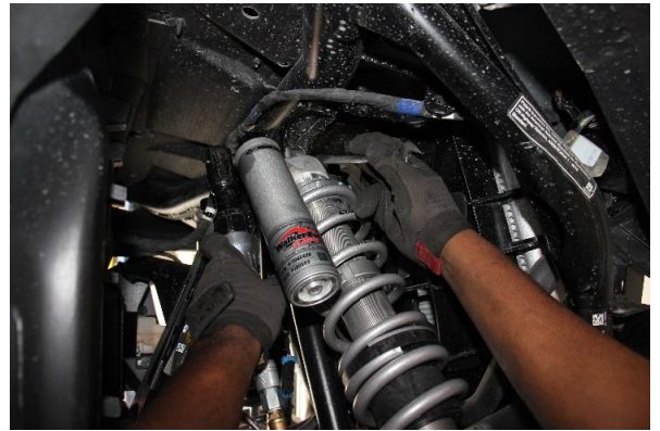
Step 16. Secure the coilover to the upper mount using the OE hardware.
