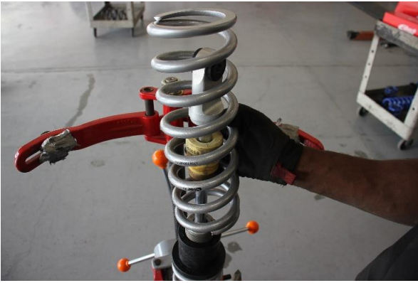
Step 13. Install the Eibach main spring.
