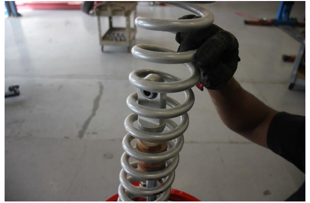
Step 14. Install the Eibach main spring.
