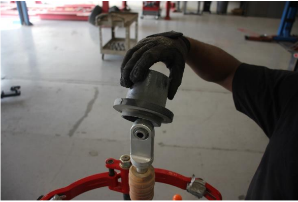
Step 7. Remove the OE slider.
