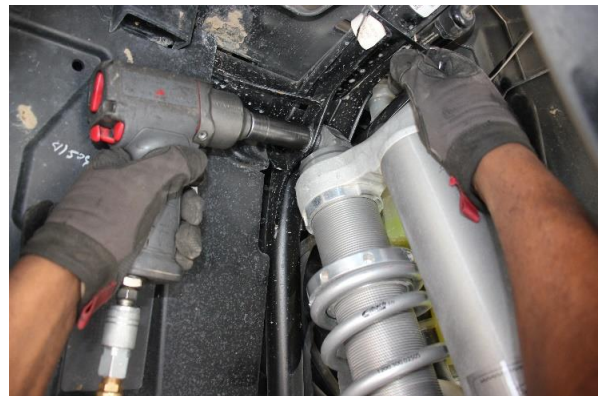
Step 18. Secure the coilover to the upper mount with the OE hardware.
