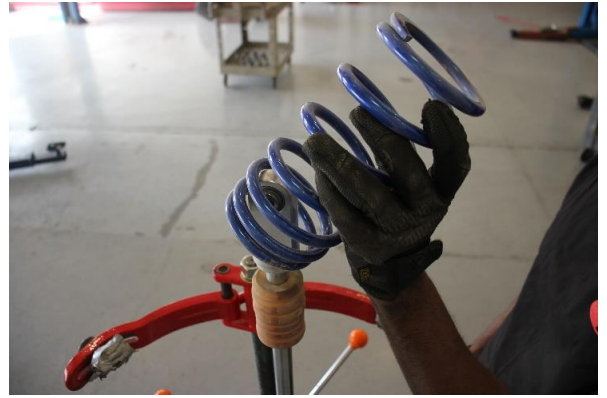
Step 8. Remove the OE secondary spring.
