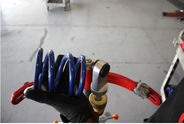
Step 7. Remove the OE secondary spring
