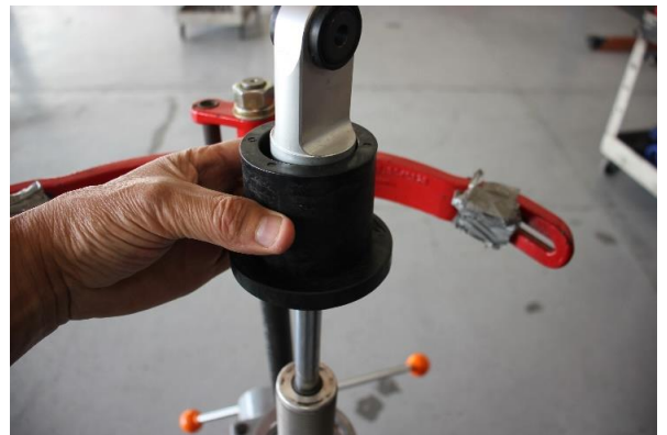
Step 12. Install the Eibach spring slider.
