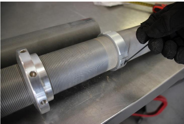
Step 11. Tighten the allen screws.
