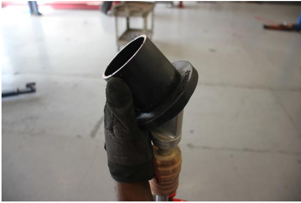
Step 13. Install the Eibach spring slider.
