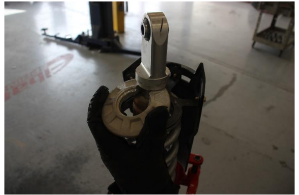
Step 16. Reinstall the factory spring retainer.
