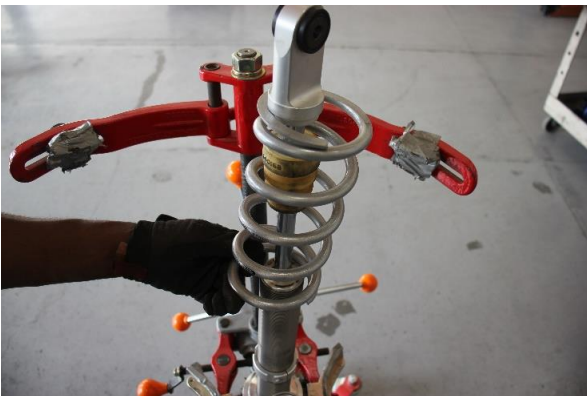
Step 11. Install the Eibach secondary spring.
