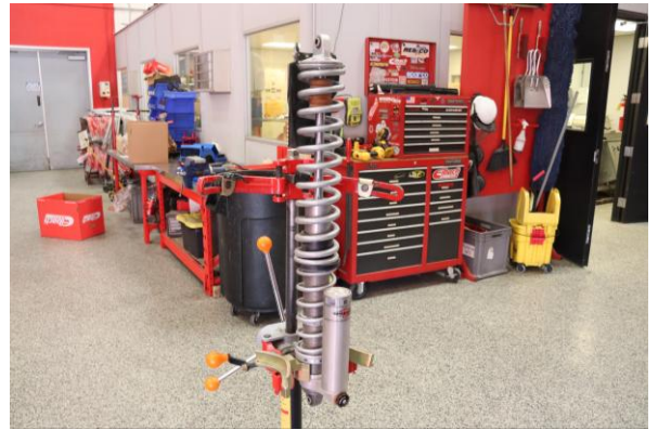
Step 22. Decompress the shock assembly ensuring the lower spring perch fully engages the lower shock mount and the plastic shield faces away from the shock reservoir.
