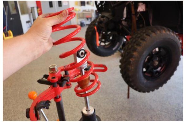
Step 8. Remove the OE main spring.
