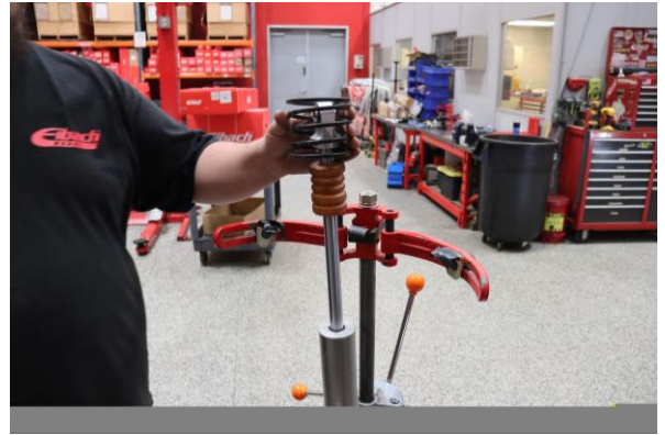
Step 14. Remove the second OE tender spring.
