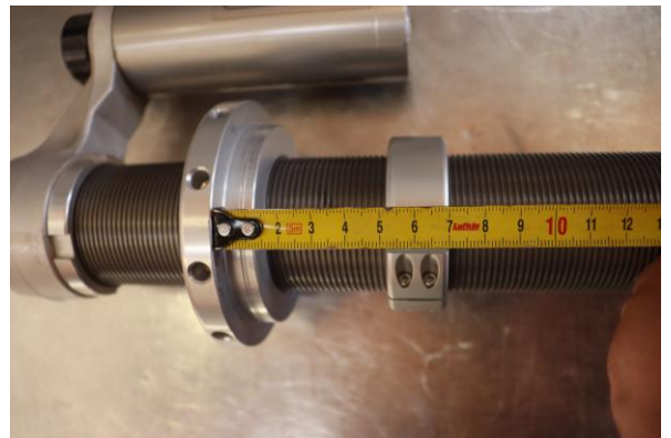
Step 12. Install Eibach crossover ring and adjust to 70mm (2 3/4 in) .
