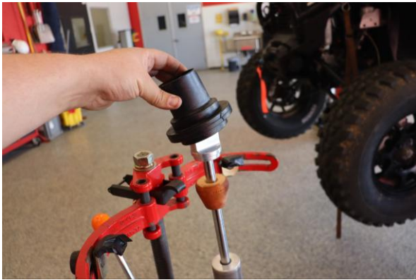
Step 9. Remove the OE spring slider.
