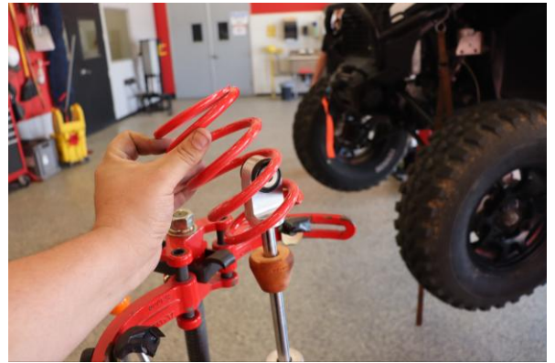
Step 10. Remove the OE tender spring.
