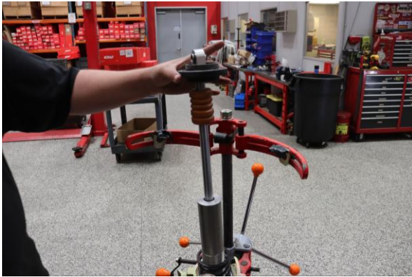
Step 13. Remove the second OE spring slider.
