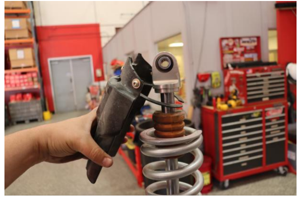
Step 20. Compress the spring assembly. Install the OE plastic shield facing away from the reservoir on the top of the assembly.
