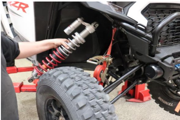
Step 17. Install shock assembly in the vehicle.
