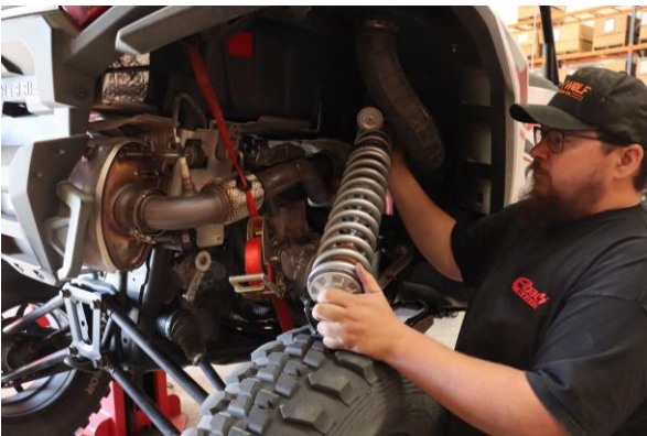
Step 23. Set the shock assembly in the vehicle.
