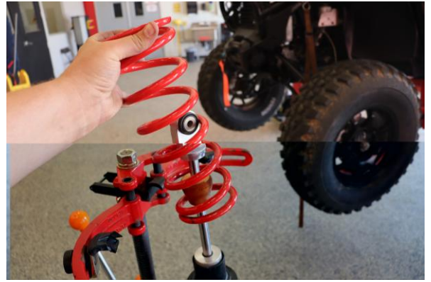
Step 8. Remove the OE main spring.
