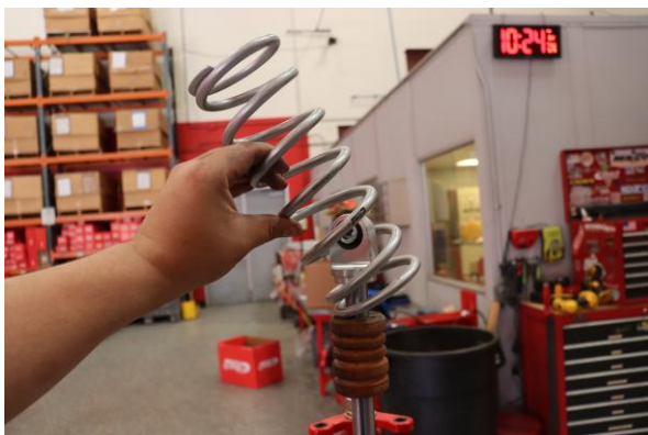
Step 17. Install Eibach tender spring.
