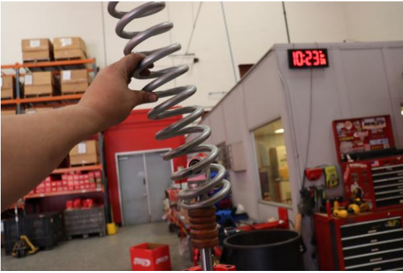
Step 19. Install Eibach main spring.
