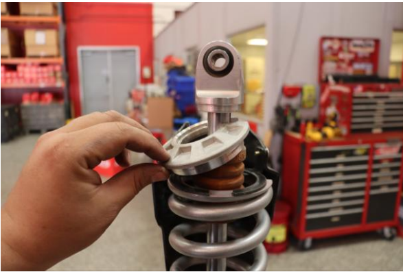
Step 21. Install the OE lower spring perch.
