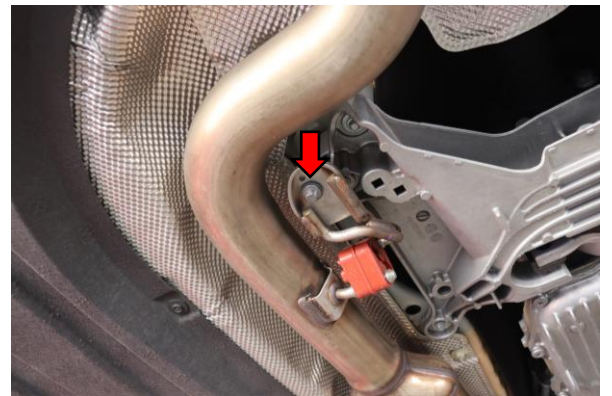
Step 36. Install forward exhaust hanger to the left of the transmission. Tighten to manufacturer specification using E12.
