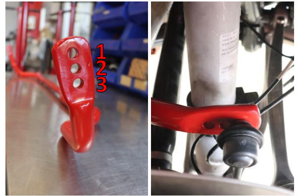
Step 28. Select a sway bar setting by installing the left and right end link into the corresponding hole on the sway bar paddle. Setting 1 provides the lowest sway bar rate, setting 3 provides the highest sway bar rate. Tighten end link to manufacturer specification using a 16mm and a T30.
