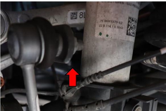
Step 17. Remove the left and right sway bar end link on the bar end using a 16mm and T30.
