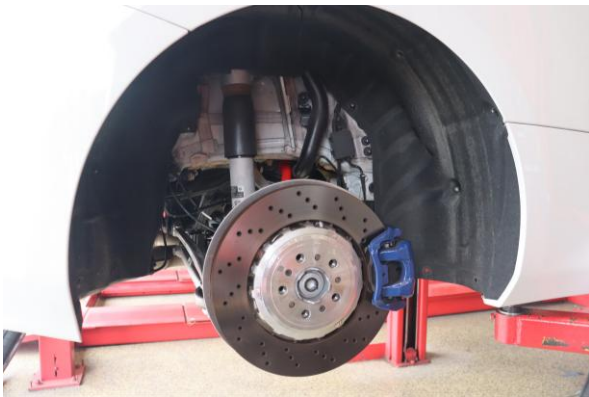
Step 39. Install both rear wheels. Tighten to manufacturer specification using a 17mm.
