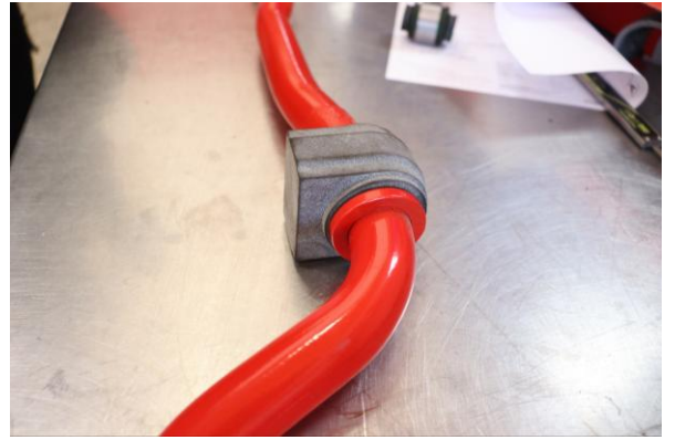
Step 20. Apply the supplied sway bar bushing grease to supplied bushing and install on sway bar inside the locating rings. Transfer both sway bar brackets from the OE sway bar.
