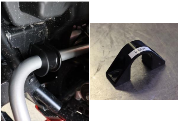
Step 5. Grease the inside of the Eibach sway bar bushings. Install Eibach sway bar brackets and bushings using supplied hardware.
