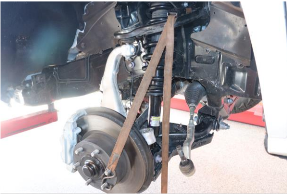
Step 9. Use a strap and secure the spindle to the frame to prevent damage to the axle CV joints.
