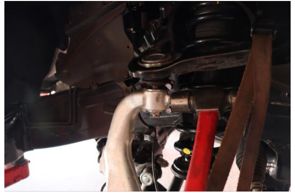
Step 8. Use a hammer against the flat portion of the spindle to shock the upper ball joint and allow it to lift out of the spindle.
