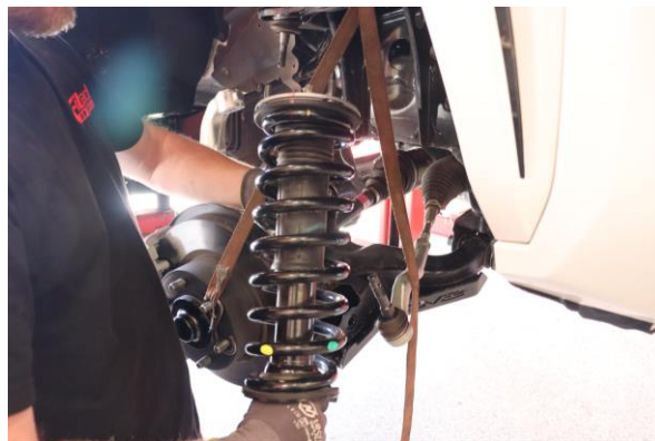
Step 13. Lower the shock assembly out down and out of the upper control arm and remove shock assembly from the truck.
