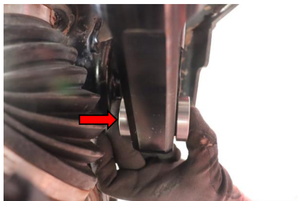
Step 15. Install the supplied spacers on either side of the lower shock bushing. The flat side of the spacer will face away from the bushing when installed correctly.
