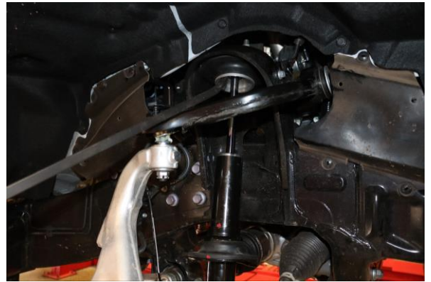
Step 10. Use a pry bar against the spring coils and the upper control arm to give the upper ball joint slack in the spindle. While holding pressure on upper control arm, remove 19mm upper ball joint. Slowly allow upper control arm to rotate up and away from spindle. Allow spindle to rest against installed strap.
