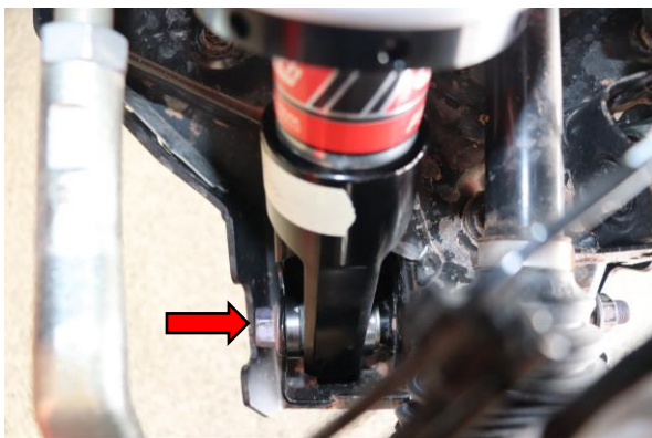
Step 16. Install the lower shock mounting bolt. Install 22mm nut on opposite side and tighten to factory specification.
