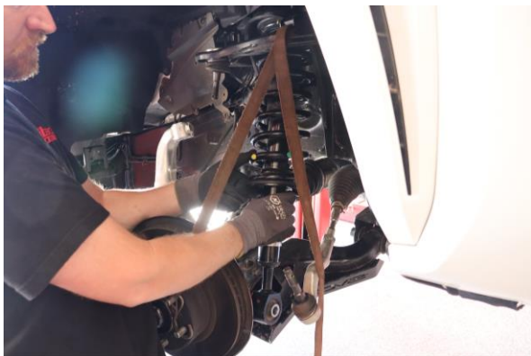
Step 12. Allow lower control arm to drop down slightly and rotate the bottom of the shock assembly toward the outside of the truck.
