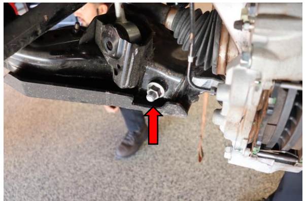
Step 11. Remove 22mm nut from lower shock mount bolt. Pull bolt from opposite side to remove.
