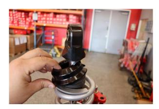
Step 21. Compress shock assembly enough to install lower spring retainer. Decompress shock and ensure spring and retainer sit flush on lower mount.
