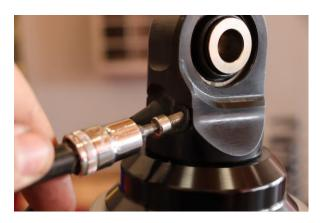
Step 22. Install lower shock wire harness in lower shock mount using both 4mm allen head screws. Tighten to manufacturer specification.
