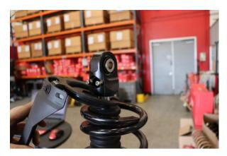
Step 11. Use a spring compressor to compress spring assembly. Remove lower spring retainer.
