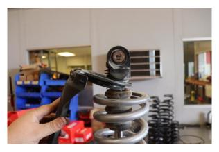
Step 20. Install lower spring retainer. Decompress spring assembly making sure that lower spring retainer and main spring sit flush with lower shock mount
