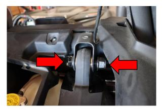
Step 8. Remove 21mm upper shock mount nut and bolt. (To remove bolt gently lift plastic trim panel to allow clearance for head of the bolt.
