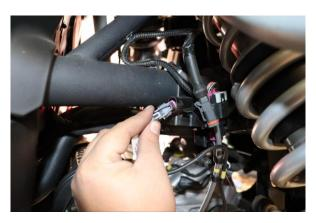
Step 26. Route the lower shock wire harness along brake line clips and connect at frame.
