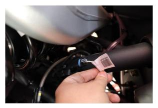
Step 2. Remove lower shock electrical connector at frame.
