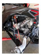
Step 1. Raise the rear of the vehicle and support it with the proper safety equipment. Remove wheel and tire. Secure trailing arm to frame using strap. **Note:**Never work on or under a vehicle that is not supported by the proper safety equipment.
