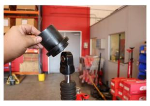
Step 19. Install OE spring slider with larger face pointed away from secondary spring.
