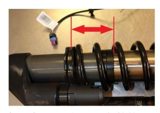
Step 17. Set crossover ring to **70mm (2 3/4in.)** from bottom of spring seat to bottom of crossover ring.
