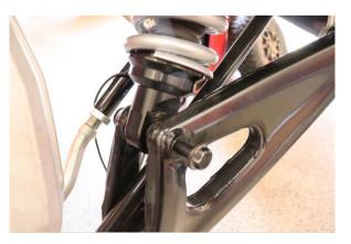
Step 24. Install lower shock bolt and tighten to manufacturer specification using 21mm socket and wrench.
