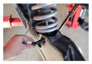
Step 7. Remove 21mm lower shock nut and bolt. (This bolt from the manufacturer has a yellow Loctite that may require a large breaker bar to remove).
