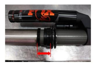
Step 16. Set crossover ring to 110mm (4 11/32in.) from bottom of spring seat to bottom of crossover ring.
