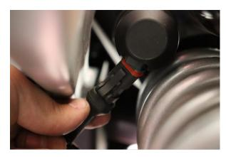
Step 27. Install the upper shock wire harness at the shock assembly.
