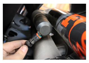
Step 25. Connect the upper shock wire harness at the shock assembly.
