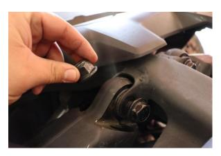
Step 24. Install upper shock mount nut and tighten to manufacturer specification using 21mm socket and wrench.
