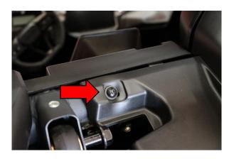
Step 6. Remove T30 screw from rear deck panel near upper shock mount.
