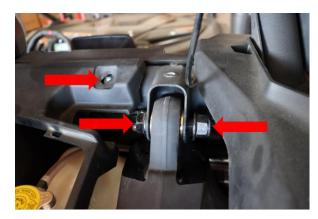
Step 23. Install upper shock mount nut and bolt. Tighten to manufacturer specification using 21mm wrench and socket. Install T30 bolt from step 6 and tighten to manufacturer specification.
