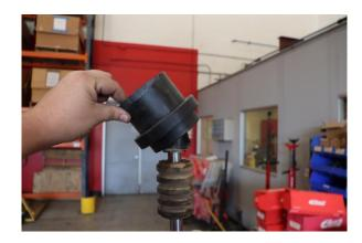
Step 18. Reinstall OE spring slider.
