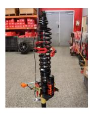
Step 12. Use spring compressor to compress shock assembly.
