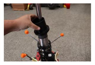
Step 14. Remove spring slider.
