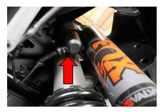
Step 5. Disconnect upper shock wire harness at shock assembly.
