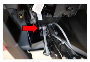
Step 2. Remove 10mm nut and T30 bolt from ride height sensor arm at front of lower trailing arm.
