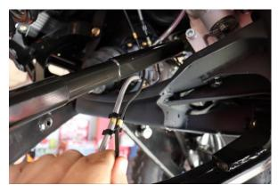
Step 3. Remove lower shock wiring harness from retaining clips along the brake line.
