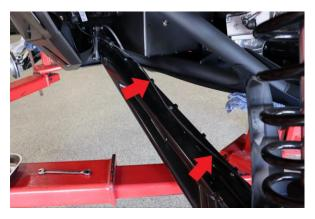
Step 3. Remove lower shock wire harness from clips along lower trailing arm.
