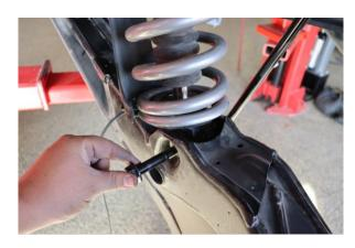
Step 24. Install lower shock mount nut and bolt. Tighten to manufacturer specification using 2 21mm sockets.
