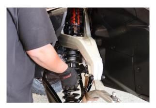
Step 10. Remove shock assembly from vehicle between upper and lower control arms.
