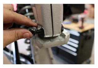
Step 25. Lower the upper control arm onto the upper ball joint and install retaining bolt. Use two 15mm sockets tighten to manufacturer specification.
