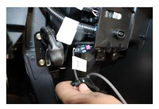
Step 4. Disconnect lower shock wire harness at front of trailing arm.
