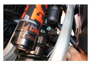
Step 4. Disconnect upper shock wiring harness at shock body.
