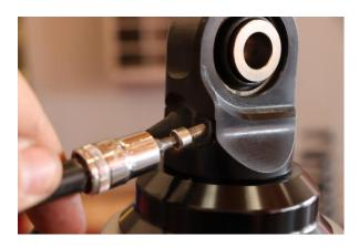
Step 11. Remove both 4mm allen head screws securing wire harness to lower shock mount. Remove wire harness from mount.
