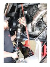
Step 9. Rotate the top of the shock assembly to the rear of the vehicle enough to clear the mount. Lift assembly from the bottom to clear the rear trailing arm and remove shock assembly from the vehicle.
