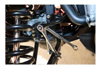
Step 6. Use 19mm wrench and 18mm socket to remove left and right sway bar end links.
