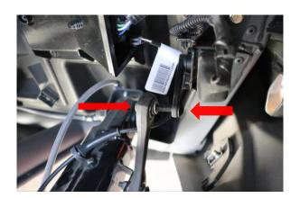
Step 28. Install ride height sensor arm at front of lower trailing arm using T30 bolt and 10mm nut. Tighten to manufacturer specification.
