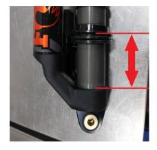
Step 16. Set pre-load spring seat to **85mm** (3 11/32in.) from bottom of seat to bottom of reservoir bridge.
