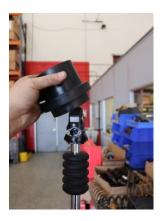
Step 13. Remove spring slider.
