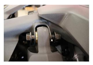
Step 9. Remove the 21mm nut and bolt from the upper shock mount. Move upper control arm up and carefully move spindle to the side.
