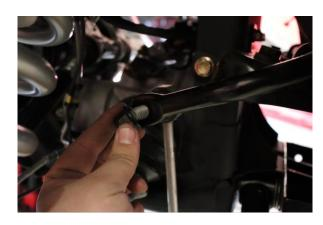
Step 28. Install sway bar end link and tighten to manufacturer specification using 19mm wrench and 18mm socket.
