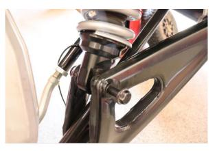
Step 8. Remove 21mm lower shock nut and bolt.
