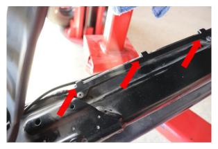
Step 26. Connect the lower shock wire harness and route through clips along lower trailing arm.
