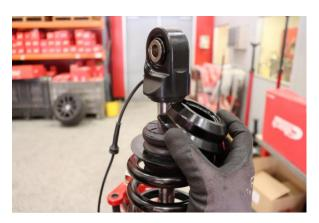
Step 12. Remove the spring retainer.
