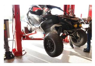
Step 1. Raise the front of the vehicle and support it with the proper safety equipment. Note: Never work on or under a vehicle that is not supported by the proper safety equipment.
