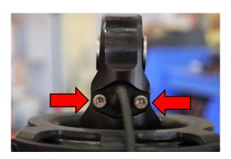
Step 10. Remove both 4mm allen head screws and disconnect lower shock wire harness.
