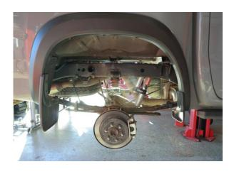
The reservoir should be mounted towards the top and pointing towards the back of the vehicle.
