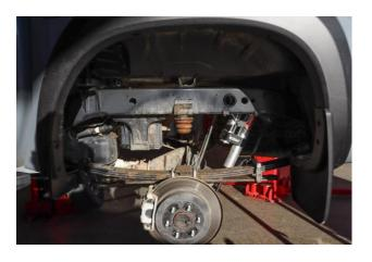
The reservoir should be mounted towards the top and pointing towards the front of the vehicle.
