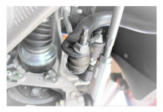
Loosen and remove factory end links
