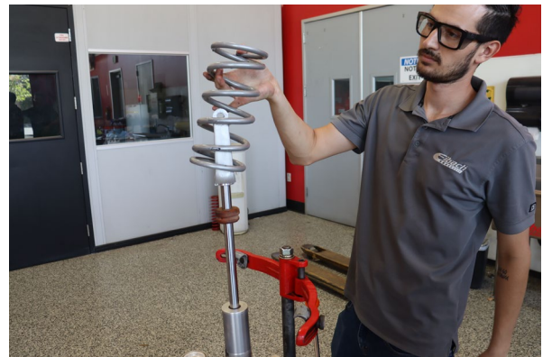
Install the Eibach Front Tender.
