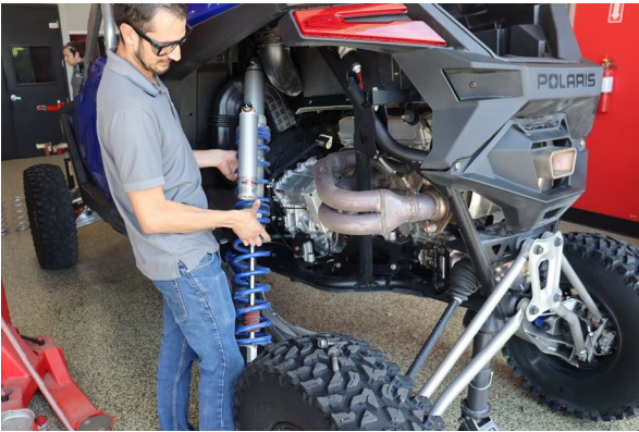
Remove the shock.
