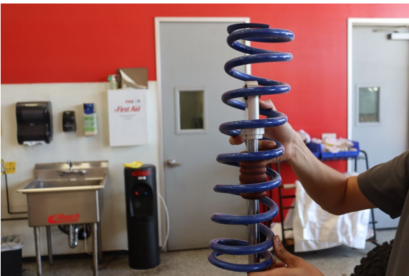
Remove the OE rear main spring.
