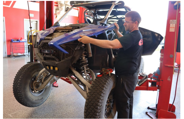
Remove the fender.
