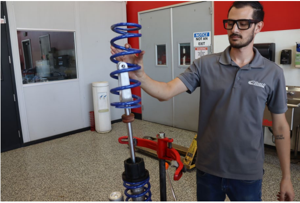
Remove the OE main spring.
