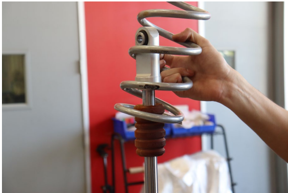
Install the Eibach rear tender spring.
