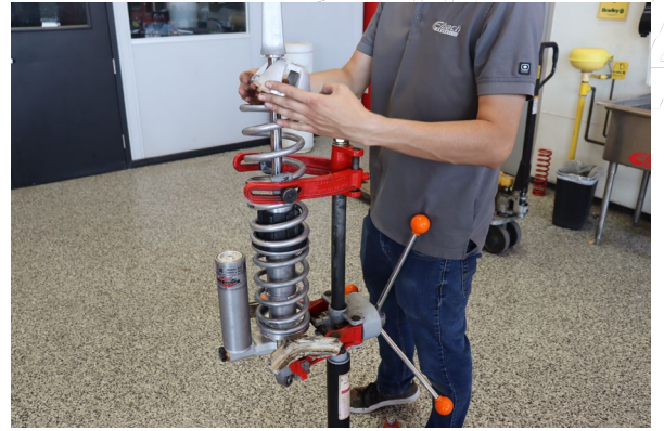
Install the Eibach main spring and the OE lower spring perch. Make sure the perch is lined up with the boss on the clevis.
