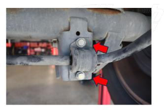
Loosen and remove OE sway bar brackets and remove sway bar.
