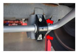
Install new bushings and brackets onto Eibach sway bar.
