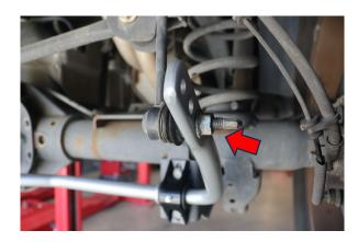
Attach factory end links to Eibach sway bar.
