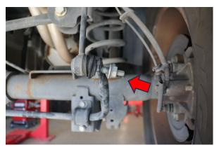
Loosen and remove OE rear end links from OE sway bar
