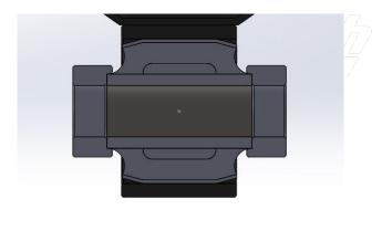
Install Bushing Spacers in the orientation as shown with the stepped side facing inwards.
