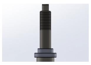
Install the Stem Spacer in the orientation as shown.
