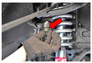
Pry down on the upper control arm, line up the upper ball joint with the knuckle, and thread on the 19mm Step 19. nut. Torque to (67 ft-lb if the holes don't line up for the clip tighten it a little more) and re install the cotter
