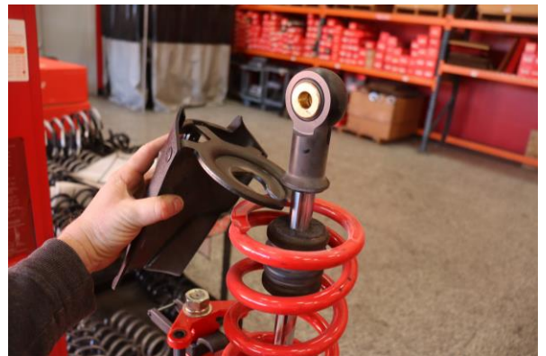
Step 28. Compress the springs and remove the OE spring seat.
