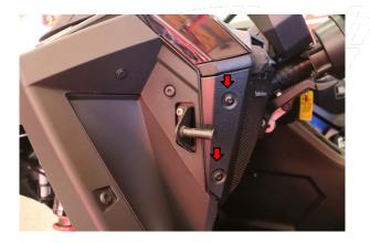
Remove the torx screws for the speaker grill
