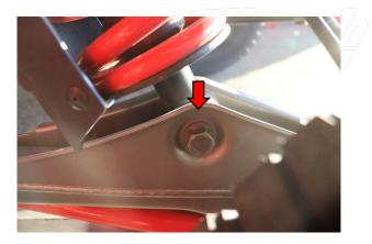
Loosen and remove the lower shock bolt.
