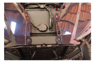
Remove the torx screws and clips securing the side hood fascia. On the passenger side the antenna will need to be removed as well.
