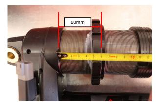
Set the preload collar to 60mm from the bottom of the Resi crossover to the bottom of the preload collar
