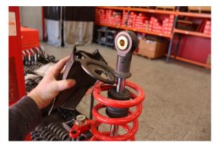
Compress the springs and remove the OE spring seat.
