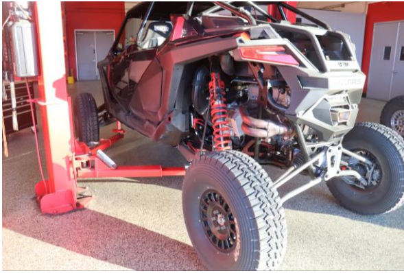
Step 23. Jack up the rear of the car so the wheels are off the ground. Loosen and remove the upper shock bolt.
