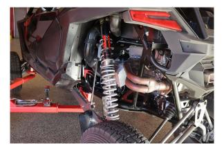
Reinstall the shock. Reconnect the electrical connectors and top and bottom bolts and repeat on the opposite side.
