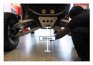
The front height should measure about 495mm from the ground to the lower control arm bolt. With a stock 32" tire. Changing tire size or extra weight will affect this measurement.
