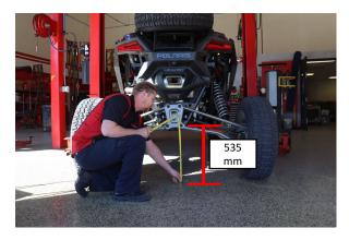
With the vehicle back on the ground, drive the car to settle the suspension and measure the height from the ground to the lower radius rod bolt. This should measure approximately 535mm with a stock 32" tire and no extra weight added. Changing tire size or adding weight will affect this measurement.
