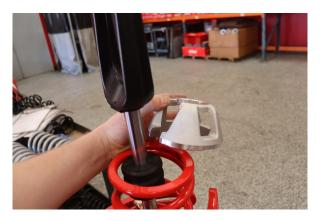
Compress the springs and remove the lower spring perch.
