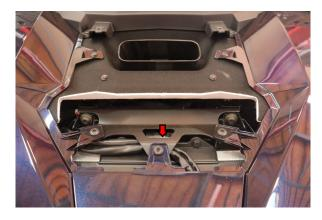
Remove the torx screw securing the front hood fascia. Push it toward the front of the car to release. For vehicles equipped with front camera unplug the harness.
