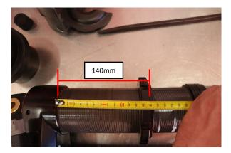
Set the preload collar to 140mm from the resi crossover bridge to the spring seat on the preload collar.
