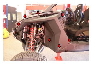
Remove all of the torx screws and clips on the fender.
