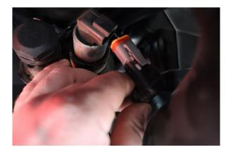
Disconnect the both electrical connectors for the Live Valve.
