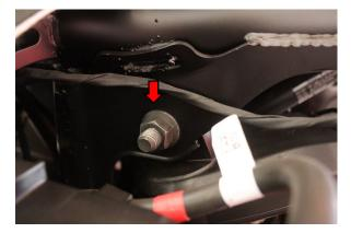
With everything removed and the car jacked up with the front wheels off the ground. Remove the upper and lower shock bolts and disconnect the electrical connectors for the Live Valve.
