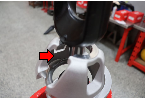
Install the OE spring perch and ensure the boss on the clevis is aligned with the opening on the perch.
