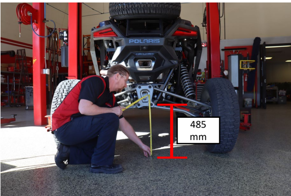
With the vehicle back on the ground, drive the car to settle the suspension and measure the height from the ground to the lower radius rod bolt. This should measure approximately 485mm with a stock 32" tire. Changing tire size or adding weight will affect this measurement.
