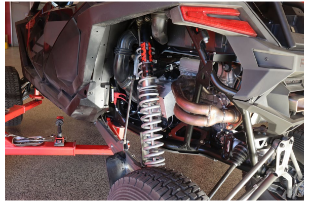
Reinstall the shock. Reconnect the electrical connectors and top and bottom bolts and repeat on the opposite side.
